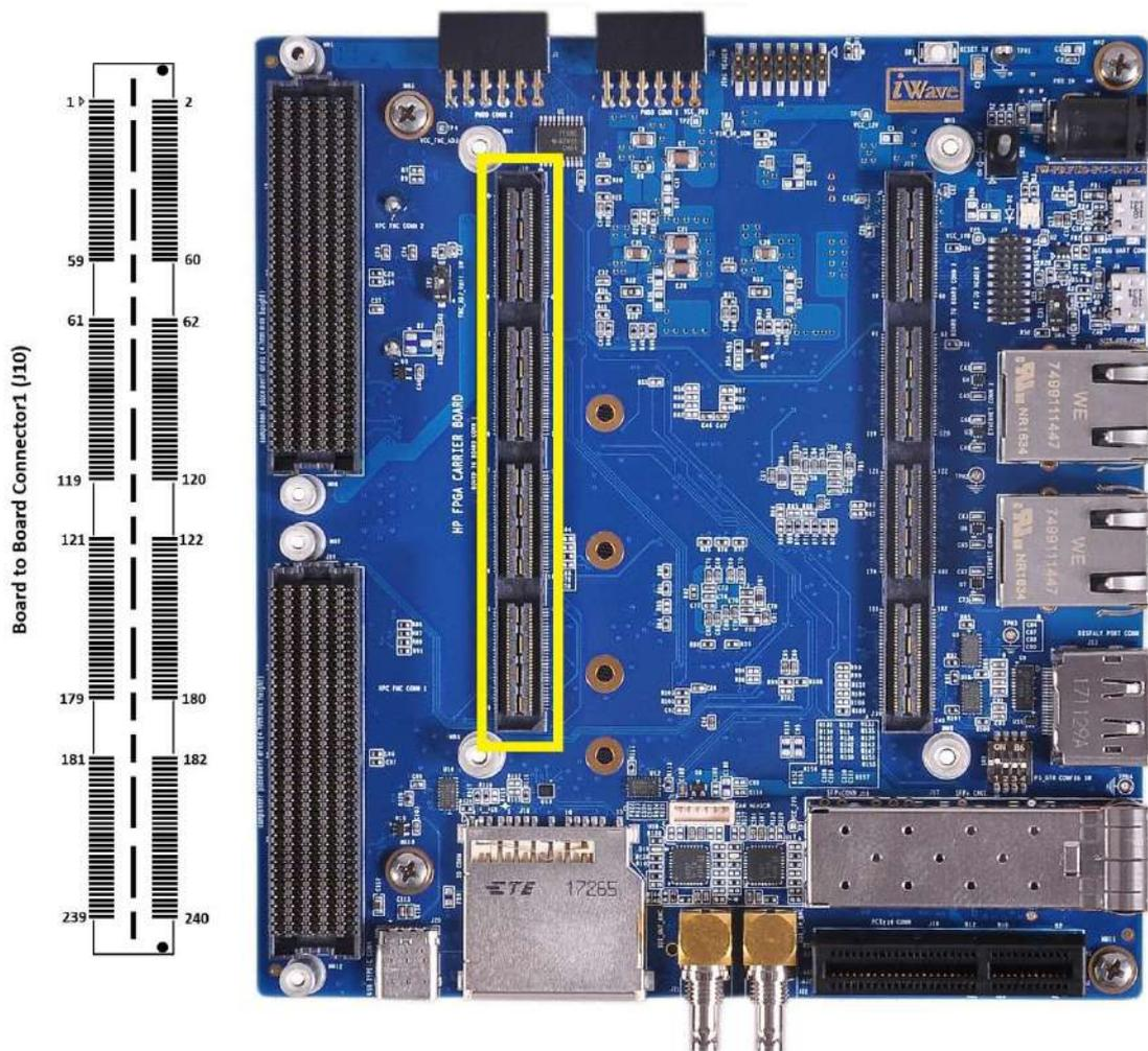
Figure 2: Board to Board Connector1
