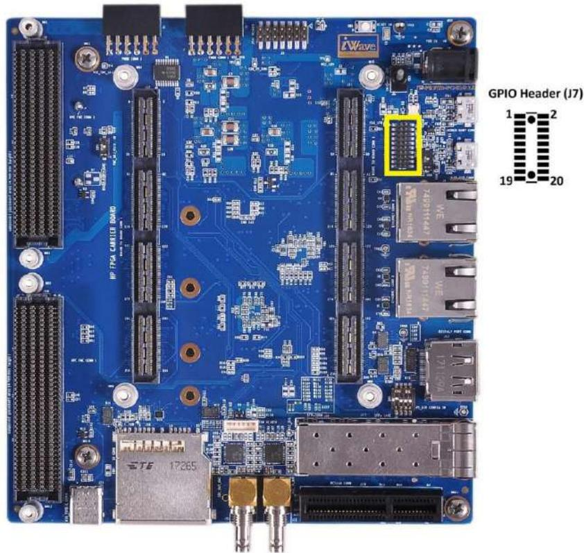
Figure 23: GPIO Header
