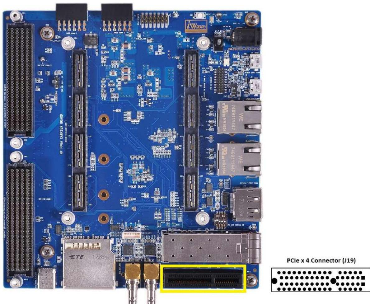
**Figure 11: PCIe x4 Connector**
