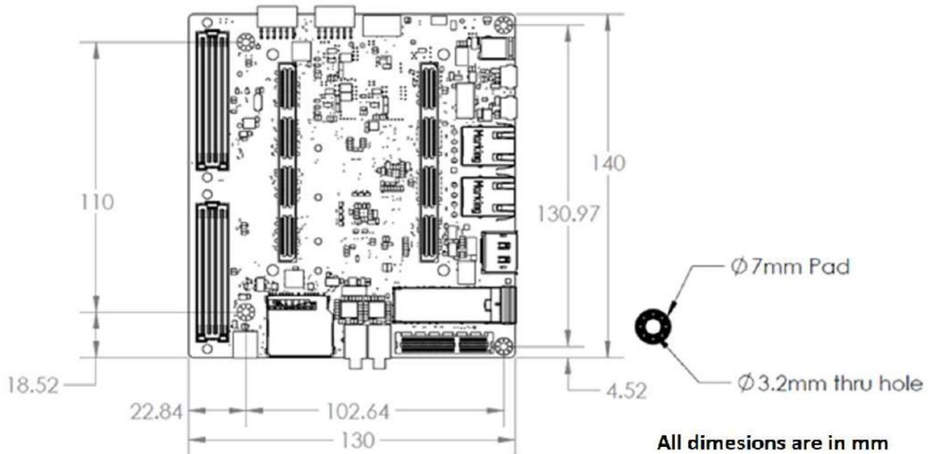
Figure 27: Carrier board Mechanical dimension – Top View
