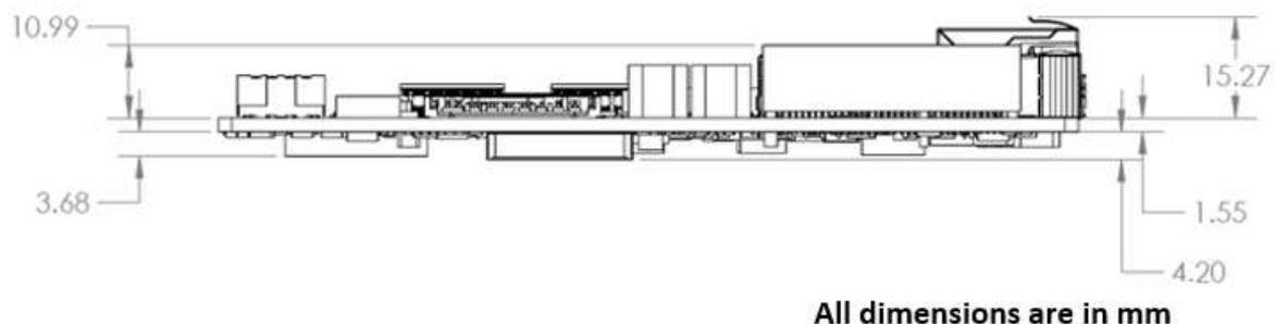
Figure 28: Carrier board Mechanical dimension – Side View
