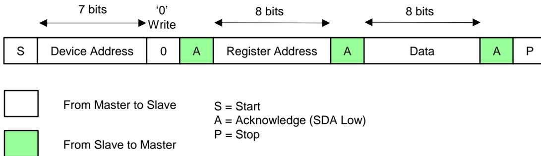
**Figure 5. I<sup>2</sup>C Write Cycle**
