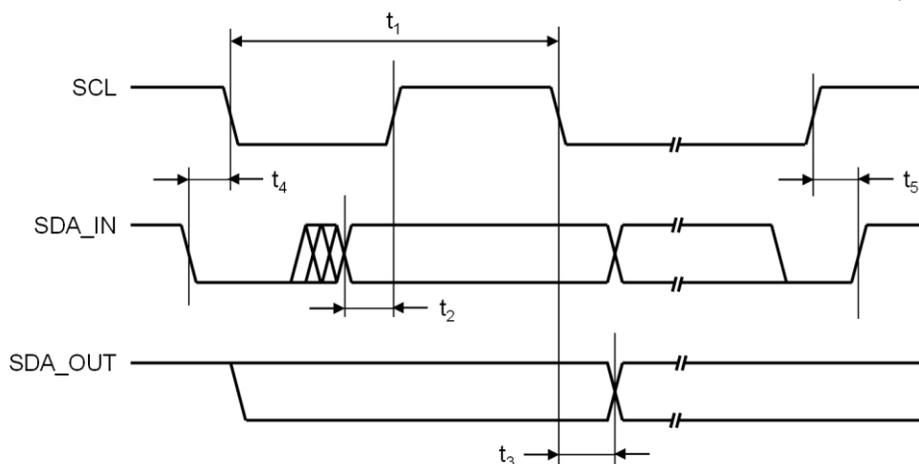
**Figure 1. I<sup>2</sup>C Compatible Interface Timing**
