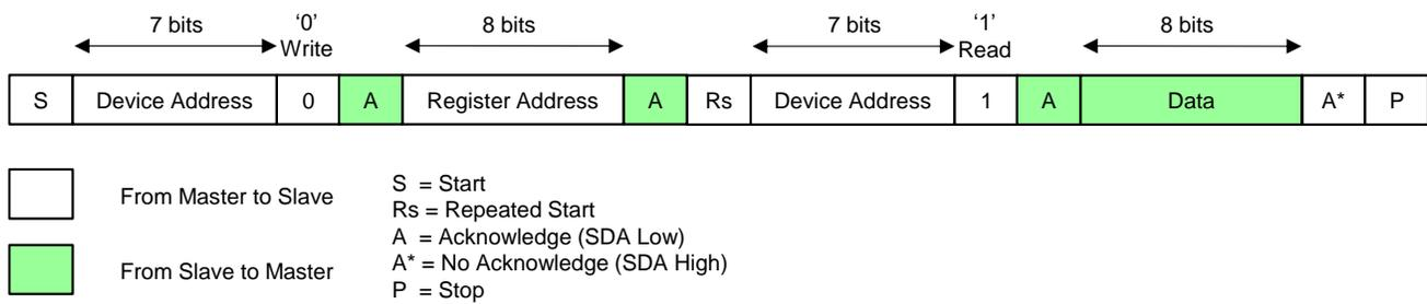
**Figure 6. I<sup>2</sup>C Read Cycle**
