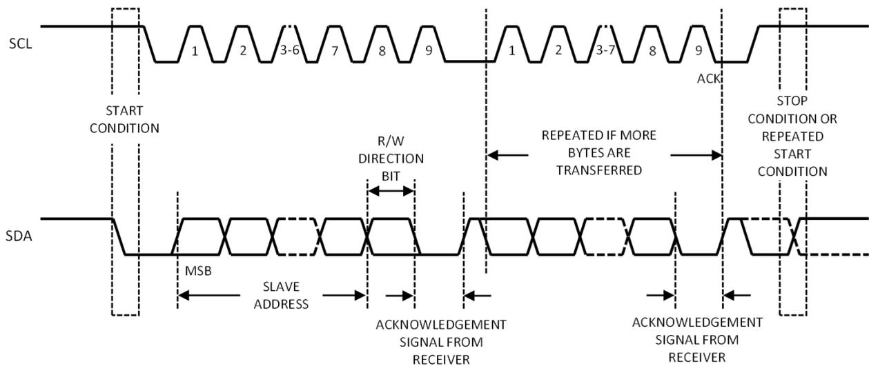
**Figure 4. Data Transfer on I<sup>2</sup>C Serial Bus**
