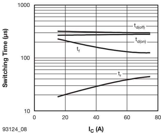
Fig. 8 - Typical IGBT Switching Time vs.  $I_C$
