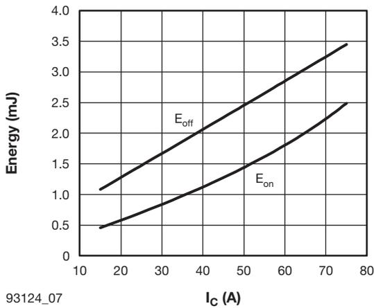
Fig. 7 - Typical IGBT Energy Loss vs.  $I_C$
