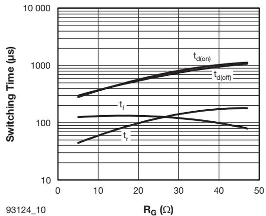
Fig. 10 - Typical IGBT Switching Time vs.  $R_G$
