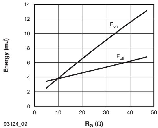
Fig. 9 - Typical IGBT Energy Loss vs.  $R_G$
