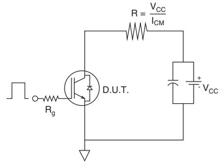
Fig. 13 - Pulsed Collector Current Test Circuit
