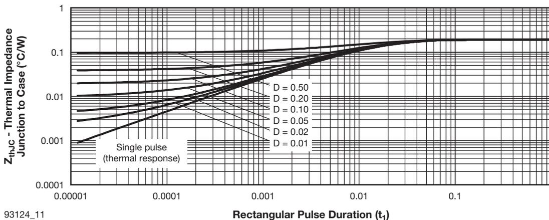
Fig. 11 - Maximum Thermal Impedance  $Z_{thJC}$  Characteristics
