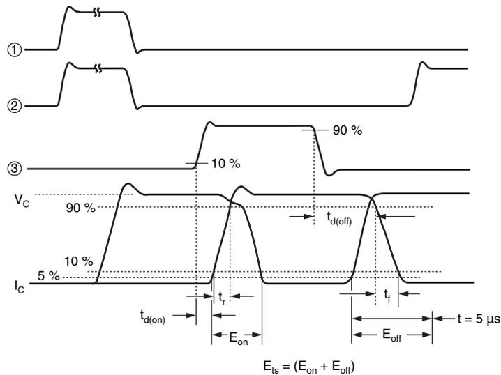
Fig. 15 - Switching Loss Waveforms Test Circuit
