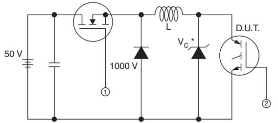
\* Driver same type as D.U.T.;  $V_C = 80\%$  of  $V_{ce(max)}$
