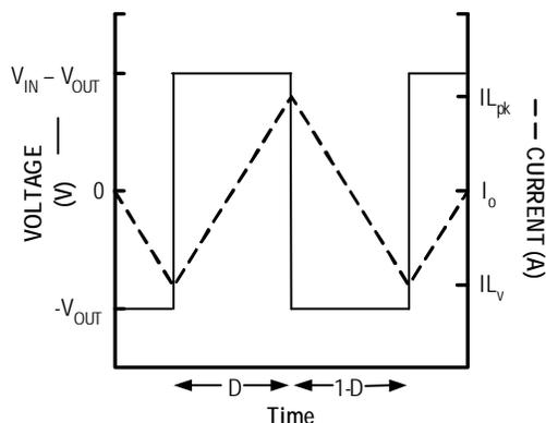
**Figure 7. Inductor Waveform**
