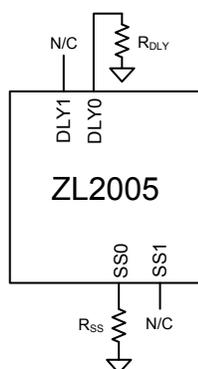
**Figure 11. DLY and SS Pin Resistor Connections**
