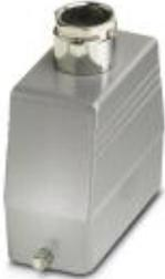
HEAVYCON sleeve housing B10, for single locking latch, height 72 mm, with screw connection 1x M25, straight conductor exit
