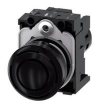
acoustic signal device, compact, 22 mm, round, plastic, black, Continuous tone 2.4 kHz, IP40, Sound pressure min. 80 dB/10 cm, with holder, Operating voltage 230 V AC, screw terminal
