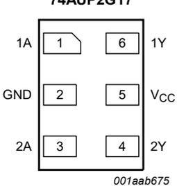
**Fig. 5. Pin configuration SOT886 (XSON6)**
