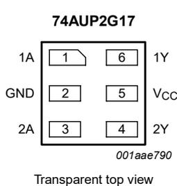
**Fig. 6. Pin configuration SOT1115 and SOT1202 (XSON6)**
