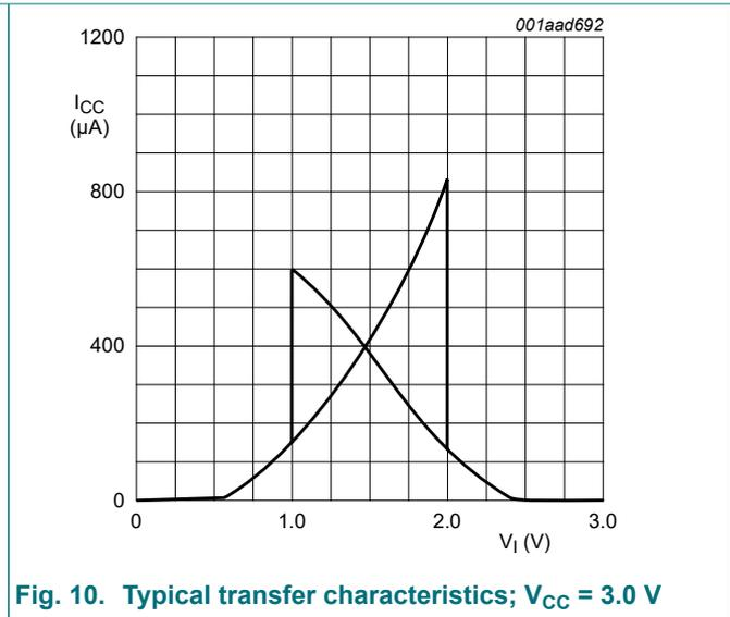
Fig. 10. Typical transfer characteristics;  $V_{CC} = 3.0\text{ V}$
