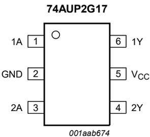
**Fig. 4. Pin configuration SOT363-2 (TSSOP6)**
