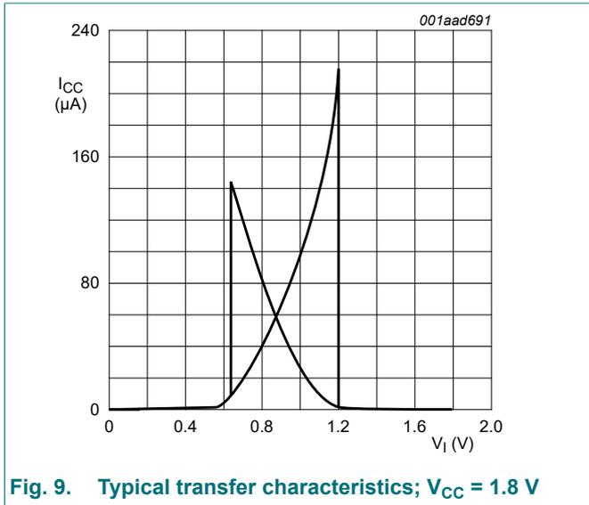
Fig. 9. Typical transfer characteristics;  $V_{CC} = 1.8\text{ V}$
