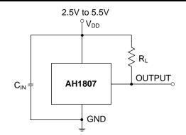
Note: 4.  $C_{IN}$  is for power stabilization and to strengthen the noise immunity, the recommended capacitance is 10nF to 100nF. R<sub>L</sub> is the pull-up resistor, the recommended resistance is 10k $\Omega$  to 100k $\Omega$ .
