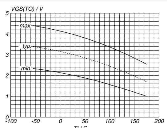
Fig.10. Gate threshold voltage.
