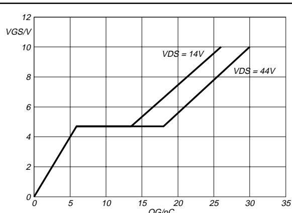
Fig.13. Typical turn-on gate-charge characteristics.
