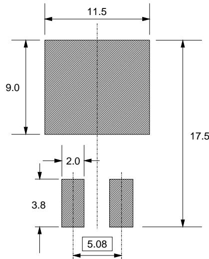
Fig.19. SOT404 : soldering pattern for surface mounting.
