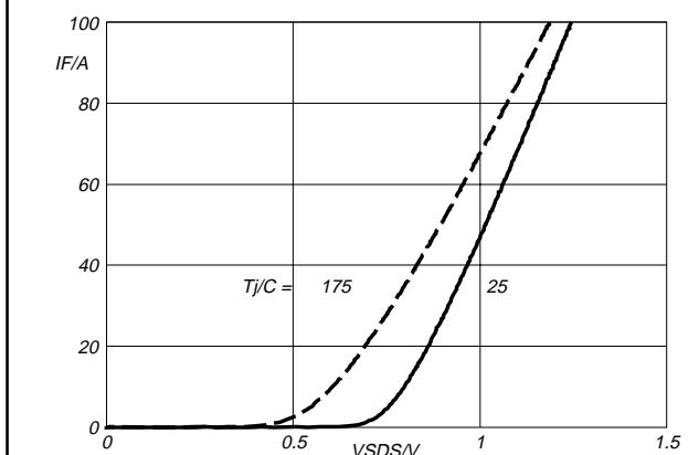
Fig.14. Typical reverse diode current.
