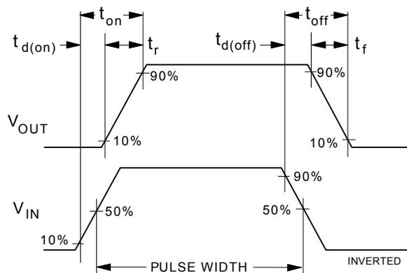
**Figure 12. Switching Waveforms.**
