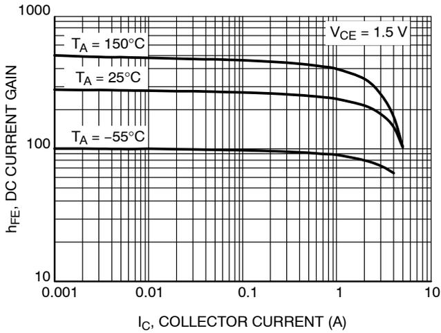
**Figure 3. DC Current Gain versus Collector Current**
