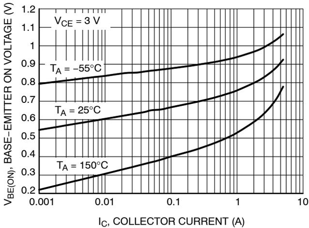
**Figure 5. Base Emitter Turn-On Voltage versus Collector Current**
