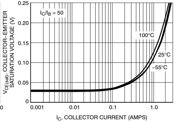
**Figure 2. Collector Emitter Saturation Voltage versus Collector Current**
