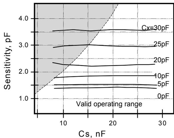
**Figure 4-3 Low Gain Sensitivity and Range @ V<sub>DD</sub> = 3V**
