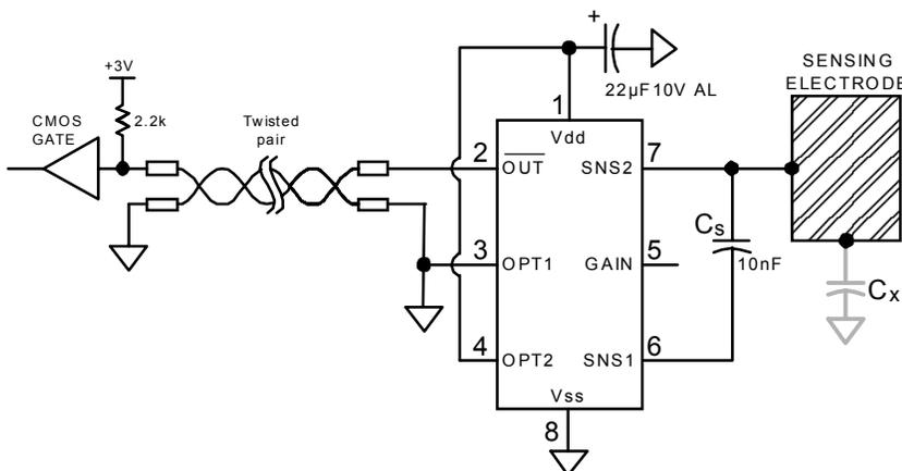
treated with caution to limit the touch area to the desired location. Multiple touch electrodes can be used, for example to create a control button on both sides of an object, however it is impossible for the sensor to distinguish between the two touch areas.
