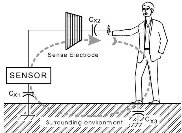
**Figure 1-6 Shielding Against Fringe Fields**
