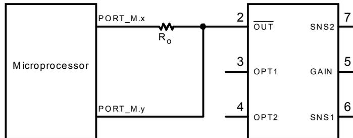
**Figure 2-5 Eliminating HB Pulses**
