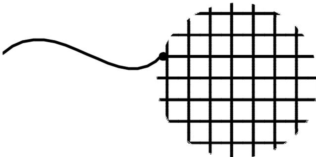
show that the electrode has more capacitance than the QT110 can tolerate, the electrode can be made into a sparse mesh (Figure 1-4) having lower  $C_x$  than a solid plane. Sensitivity may even remain the same, as the sensor will be operating in a lower region of the gain curves.
