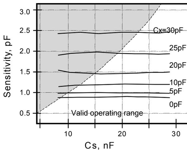
**Figure 4-2 Medium Gain Sensitivity and Range @ V<sub>DD</sub> = 3V**
