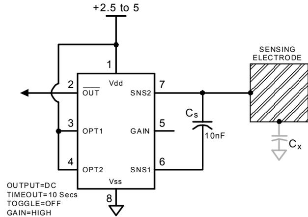
The IC is highly tolerant of changes in  $C_s$  since it computes the threshold level ratiometrically with respect to absolute load, and does so dynamically at all times.
