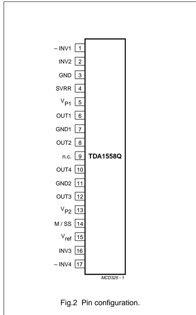
Fig.2 Pin configuration.
