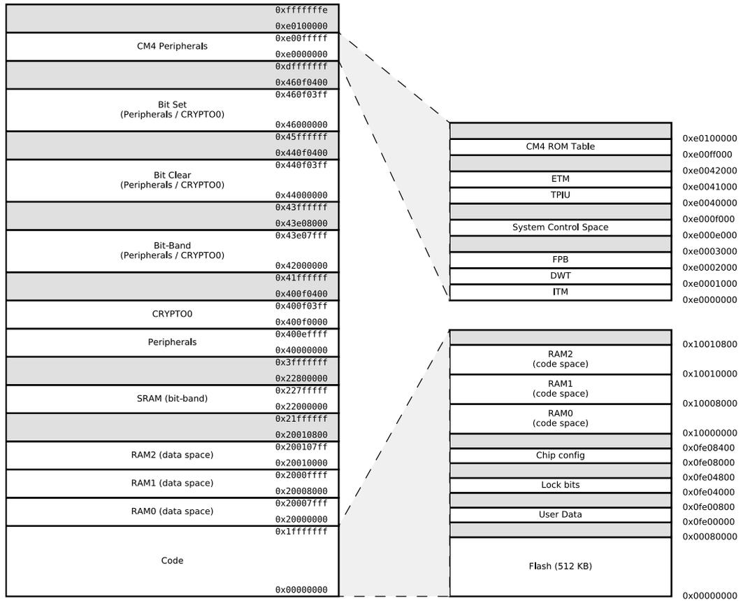
Figure 3.2. EFR32MG13 Memory Map — Core Peripherals and Code Space
