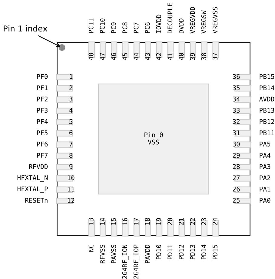
Figure 6.2. QFN48 2.4 GHz Device Pinout
