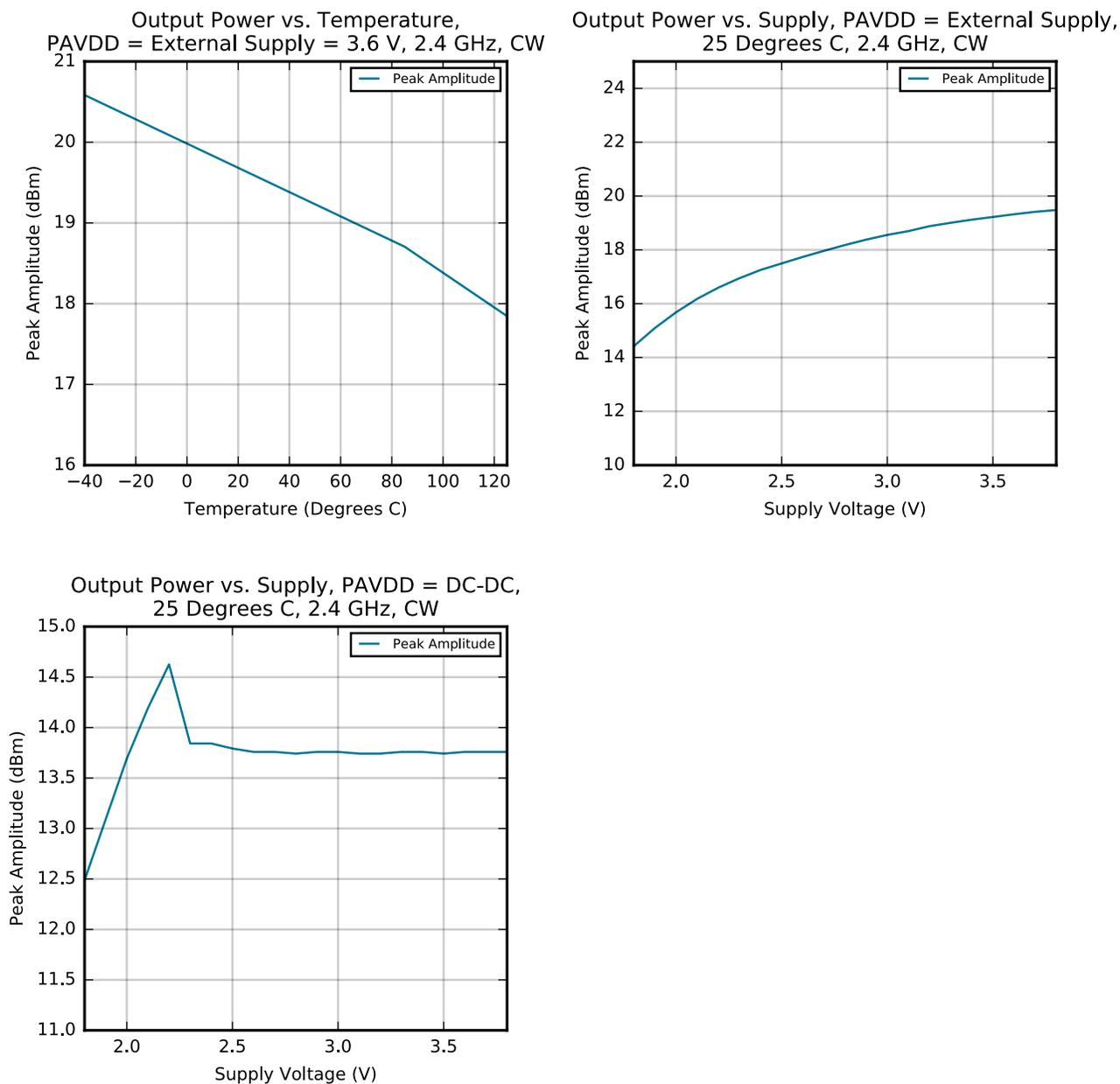
Figure 4.11. 2.4 GHz RF Transmitter Output Power
