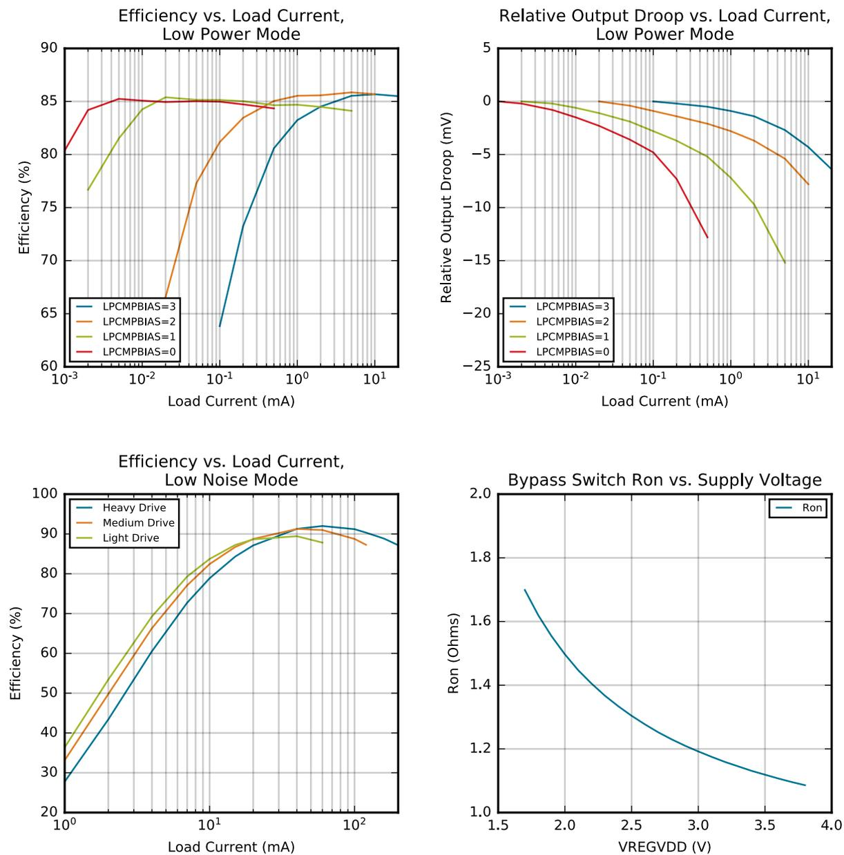
Figure 4.9. DC-DC Converter Typical Performance Characteristics
