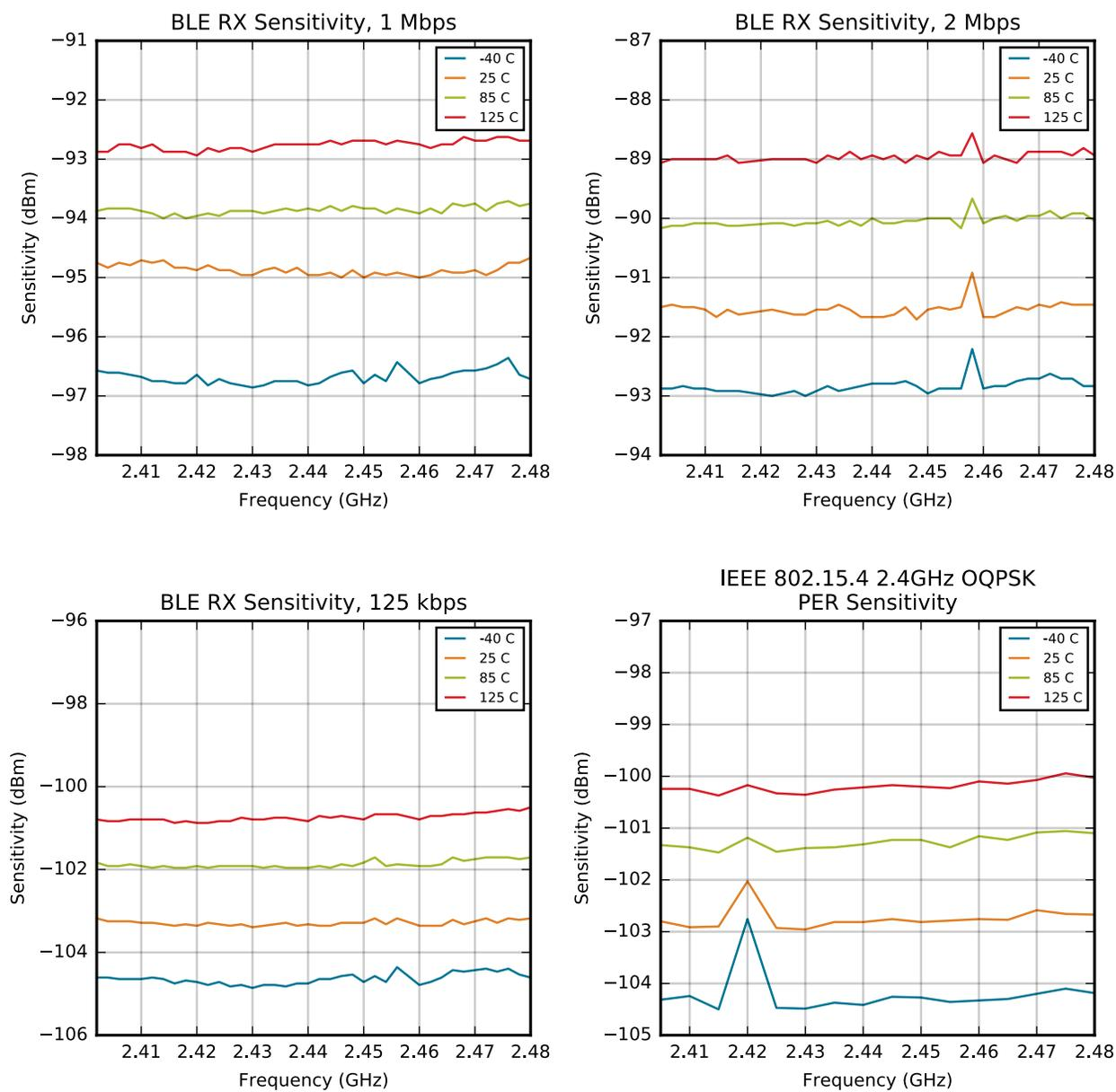
Figure 4.12. 2.4 GHz RF Receiver Sensitivity
