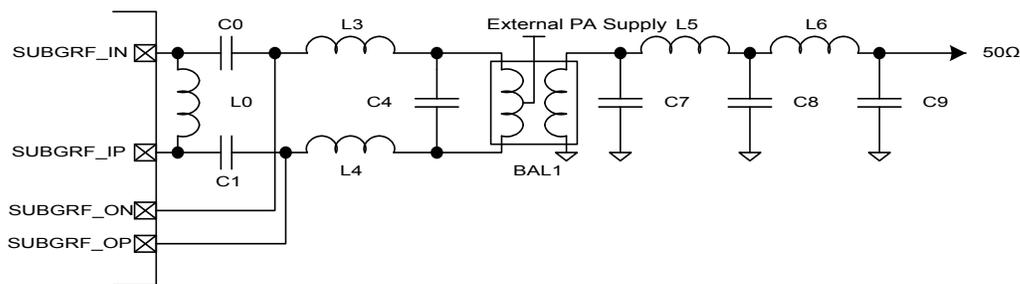
**Figure 5.5. Typical Sub-GHz RF impedance-matching network circuits**
