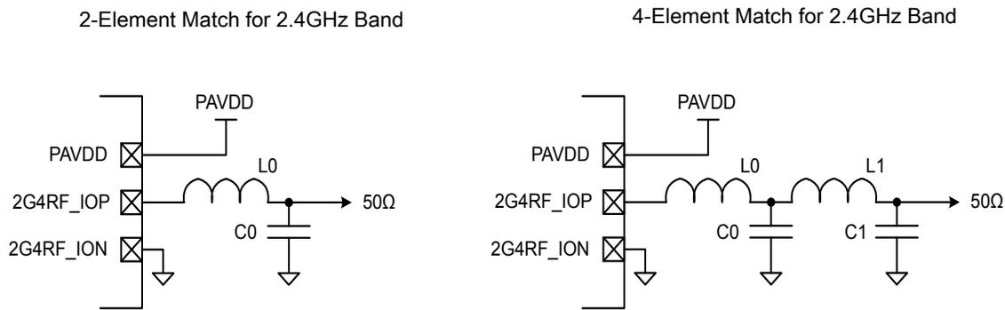
**Figure 5.4. Typical 2.4 GHz RF impedance-matching network circuits**
