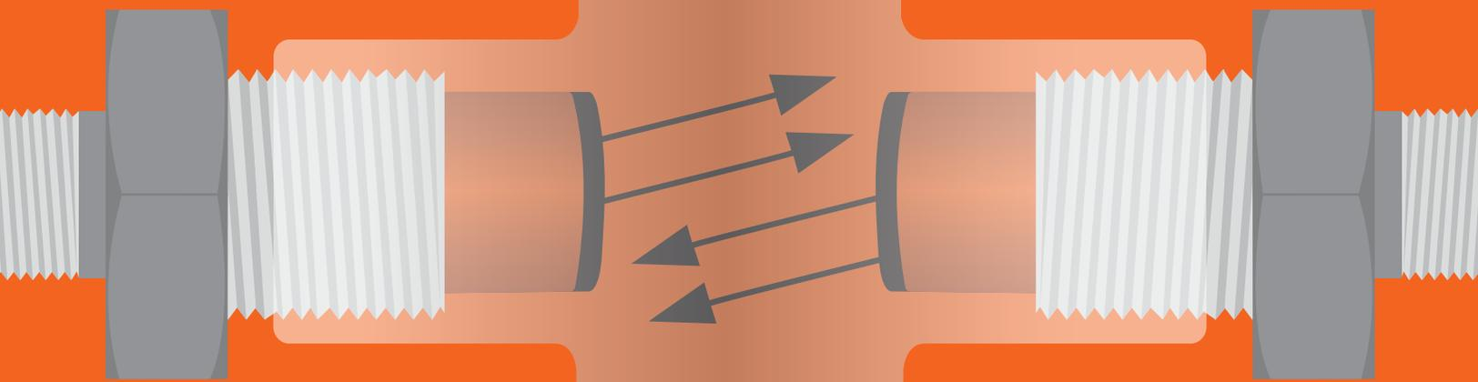
**This CO2 sensor emits a small amount of IR light; the opposing sensor will detect that light. Over several hours the CO2 readings will become unstable and take on a sine wave appearance.**
