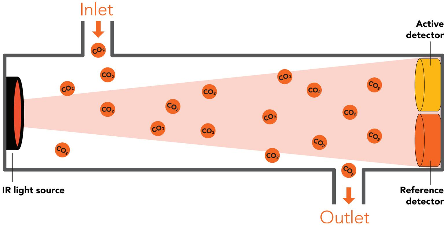
Gaseous CO<sub>2</sub> has a prominent absorption band centered at 4.2µm. CO<sub>2</sub> content is derived by quantifying how much light energy has been lost when it travels through a gaseous matrix over a fixed distance.
