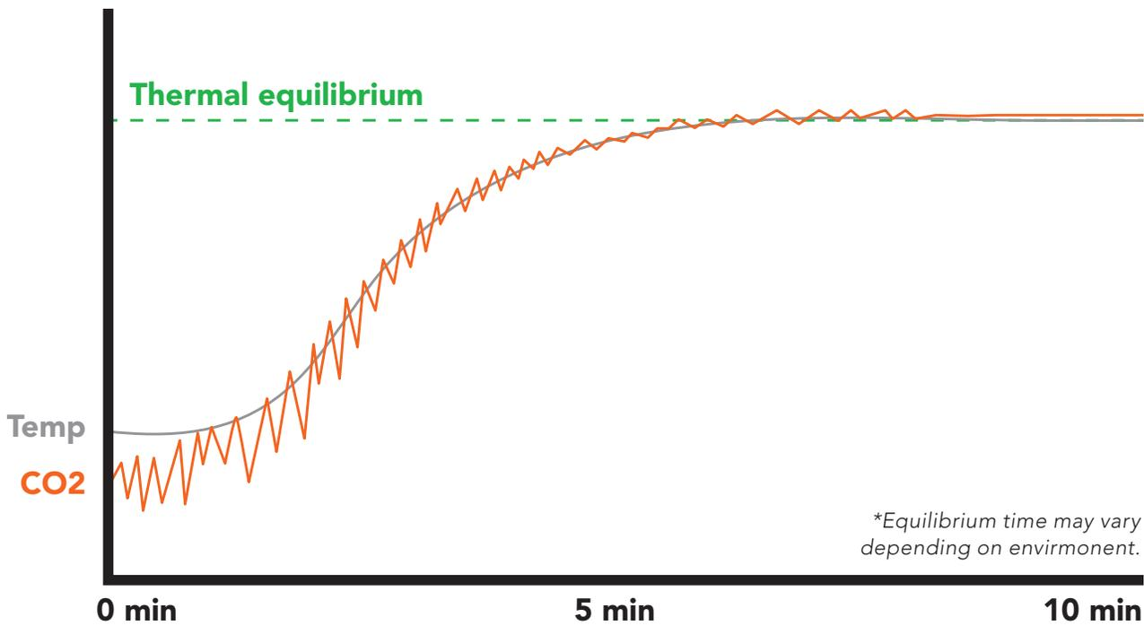
To see the internal temperature of the sensor and watch as it stabilizes, use the 'O' command found on page 25.
