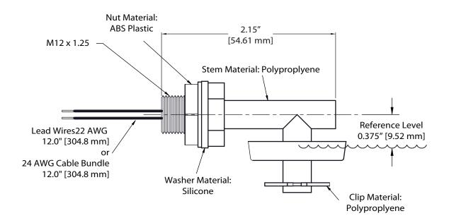
The 90-degree float switch design eliminates the problems often encountered with typical "pivot type" side-mounted float switches. The FH-VIW is available with 5 or 50-watt switching capabilities and optional Buna floats are available for oils and other low specific gravity float switch applications. Because horizontal sensors come as standard parts or customized OEM, it can be used in a vast amount of applications in many markets at a reasonable prices.
