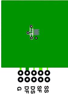
a) 50°C/W when mounted on a 1 in<sup>2</sup> pad of 2 oz copper.
