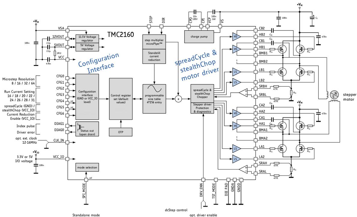
Figure 1.2 TMC2160 standalone driver application diagram
