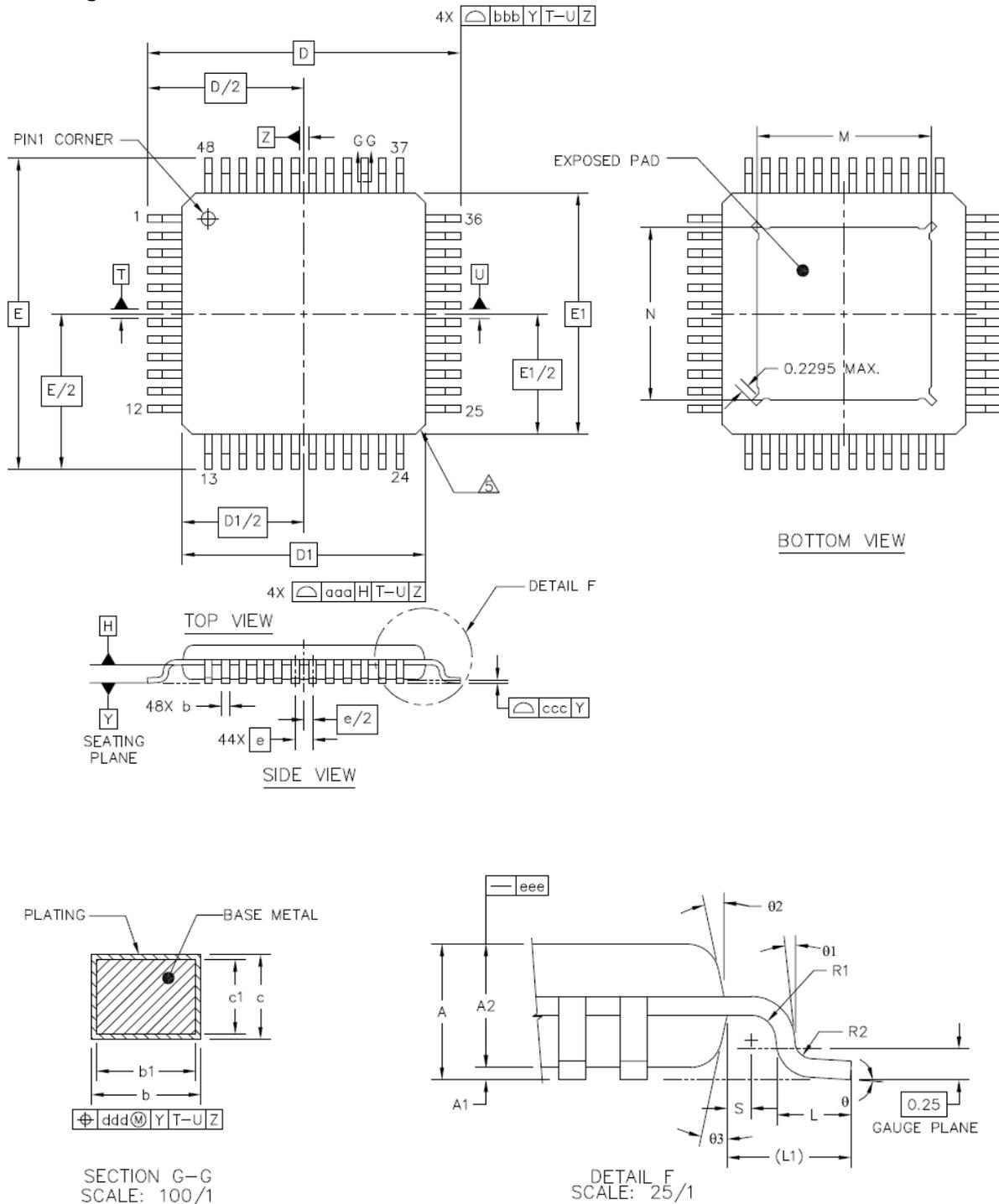
Figure 26.1 Dimensional drawings TQFP48-EP
