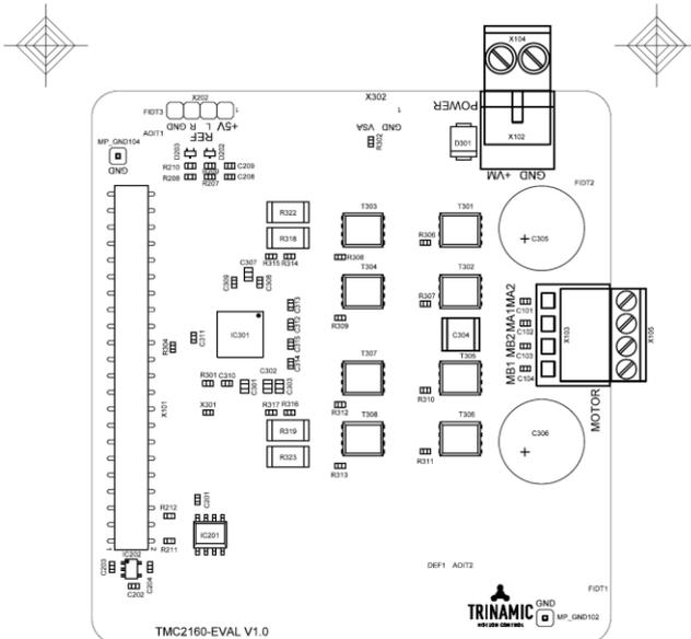
The TMC2160-EVAL is part of TRINAMICs universal evaluation board system which provides a convenient handling of the hardware as well as a user-friendly software tool for evaluation. The TMC2160 evaluation board system consists of three parts: LANDUNGSBRÜCKE (base board), ESELSBRÜCKE (connector board including several test points), and TMC2160-EVAL.
