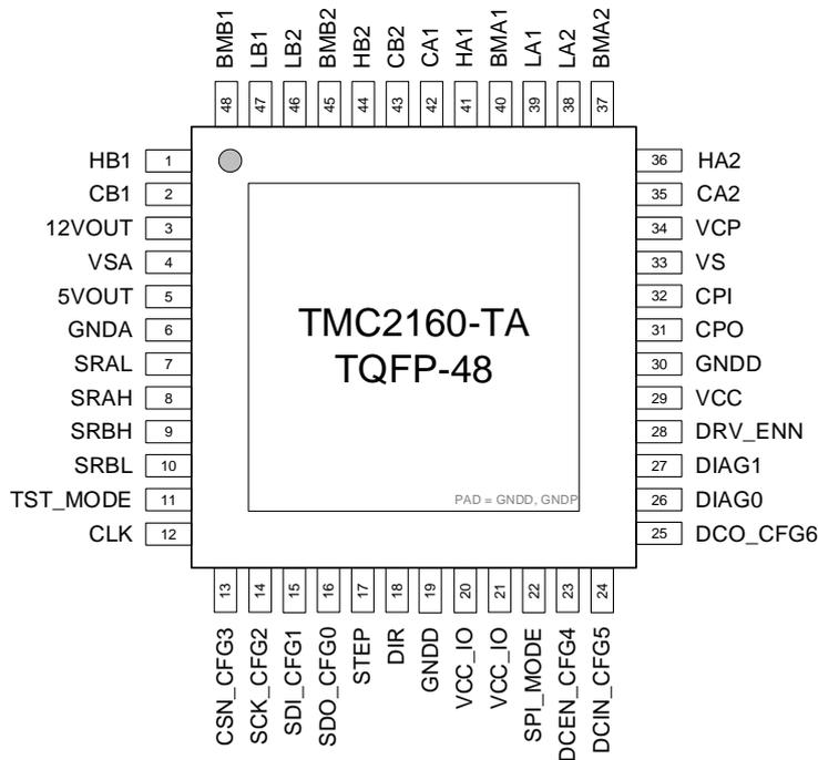
Figure 2.1 TMC2160-TA package and pinning TQFP-EP 48 (7x7mm<sup>2</sup> body, 9x9mm<sup>2</sup> with leads)
