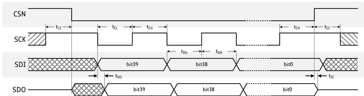
**Figure 4.1 SPI timing**
