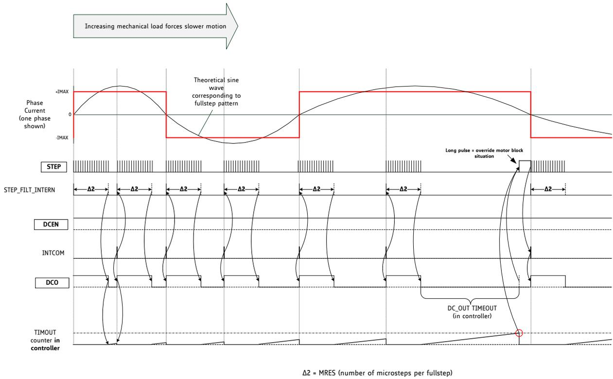
Figure 15.4 DCO Interface to motion controller – step generator stops when DCO is asserted
