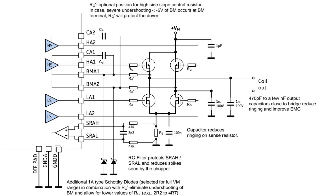
Decide use and value of the additional components based on measurements of the actual circuit using the final layout!
