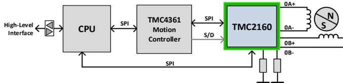
The CPU initializes the TMC4361 motion controller and the TMC2160. Thereafter, it sends target positions to the TMC4361. Now, the TMC4361 takes control over the TMC2160. Combining the TMC4361 and the TMC2160 offers diverse possibilities for demanding applications including servo drive features.
