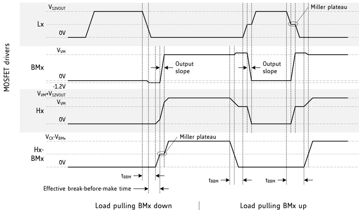
**Figure 3.4 Slopes, Miller plateau and blank time**
