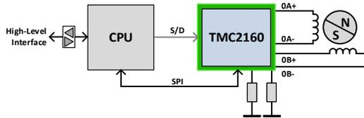
In this application, the CPU initializes the TMC2160 motor driver via SPI interface and controls motor movement by sending step and direction signals. A real time software realizes motion control.
