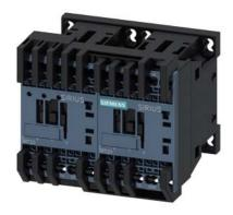
Reversing contactor assembly for 3RA27 AC-3, 4 kW/400 V, 24 V DC 3-pole, Size S00 Spring-type terminal electrical and mechanical interlock with voltage tap
