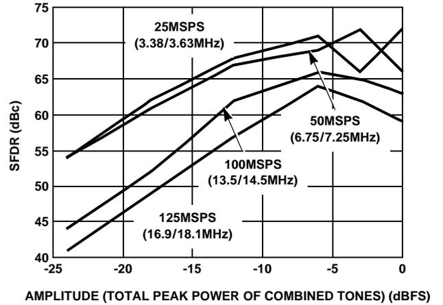
FIGURE 8. SFDR vs AMPLITUDE OF TWO TONES,  $f_{CLK}/f_{OUT} = 7$
