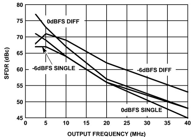
FIGURE 29. DIFFERENTIAL vs SINGLE-ENDED, CLOCK = 100MSPS
