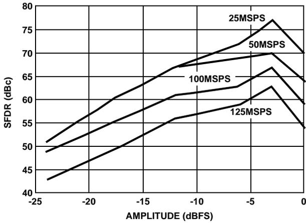
FIGURE 7. SFDR vs AMPLITUDE,  $f_{CLK}/f_{OUT} = 5$
