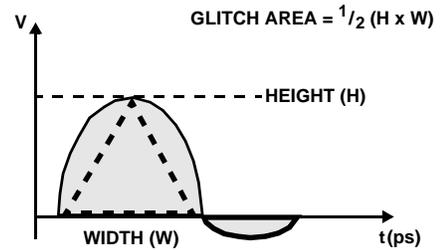
FIGURE 40. PEAK GLITCH AREA (SINGLET) MEASUREMENT METHOD
