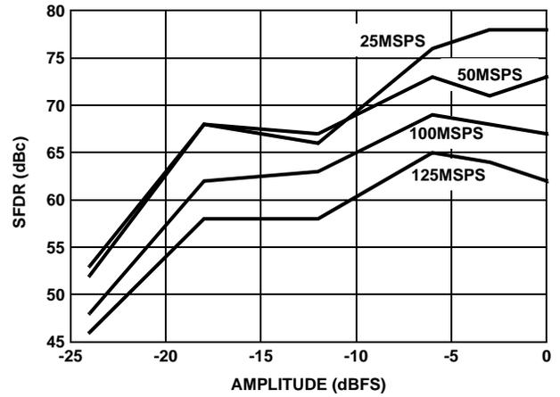
FIGURE 25. SFDR vs AMPLITUDE,  $f_{CLK}/f_{OUT} = 10$
