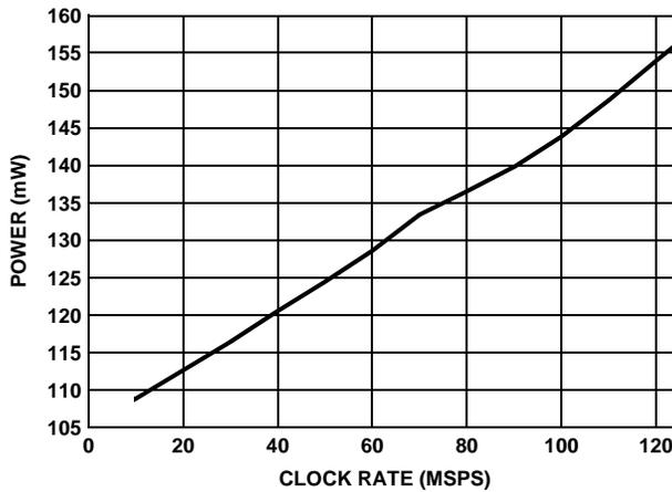
FIGURE 19. POWER vs CLOCK RATE,  $f_{CLK}/f_{OUT} = 10$ ,  $I_{OUT} = 20mA$
