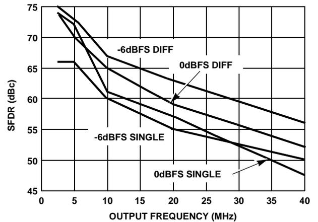
FIGURE 10. DIFFERENTIAL vs SINGLE-ENDED, CLOCK = 100MSPS
