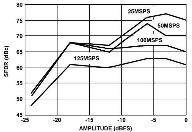
FIGURE 6. SFDR vs AMPLITUDE,  $f_{CLK}/f_{OUT} = 10$
