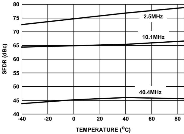
FIGURE 30. SFDR vs TEMPERATURE, CLOCK = 100MSPS
