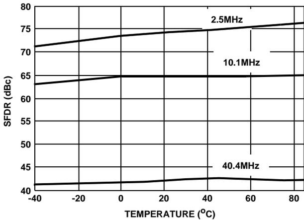
FIGURE 11. SFDR vs TEMPERATURE, CLOCK = 100MSPS
