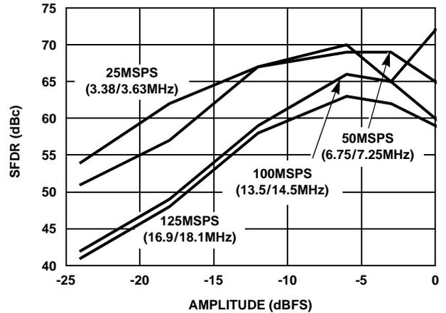
FIGURE 27. SFDR vs AMPLITUDE OF TWO TONES,  $f_{CLK}/f_{OUT} = 7$
