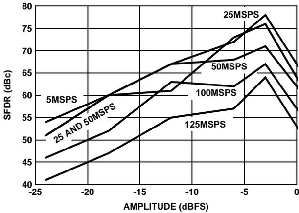
FIGURE 26. SFDR vs AMPLITUDE,  $f_{CLK}/f_{OUT} = 5$
