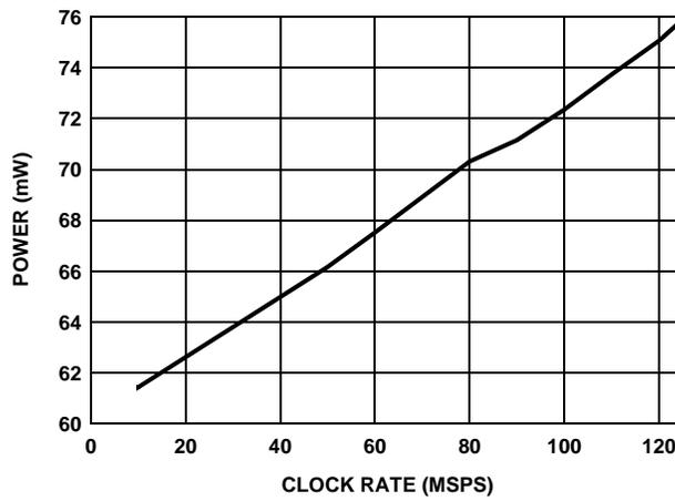
FIGURE 38. POWER vs CLOCK RATE,  $f_{CLK}/f_{OUT} = 10$ ,  $I_{OUT} = 20mA$
