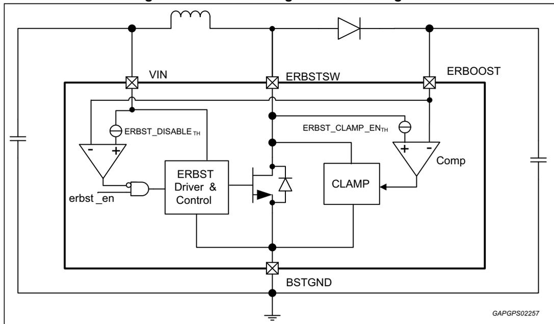
Normal run time power for the system is provided directly from the battery input, not from the boost. Boost energy is available to the system through the energy reserve crossover switch once battery is lost or a commanded system shutdown is initiated.
