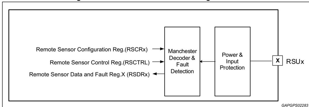
Remote sensor configuration can be addressed via the Remote Sensor Configuration Registers (RSCRx). Some of the bit fields in the RSCRx registers are available depending on the chosen configuration, remote sensor rather than wheel speed sensors. In particular, TSxDIS bit allows overriding the time slot control for PSI5 I/F and BLKTxSEL allows selection between 5ms and 10ms for the blanking time applied to the current limitation fault detection each time a channel is activated.
