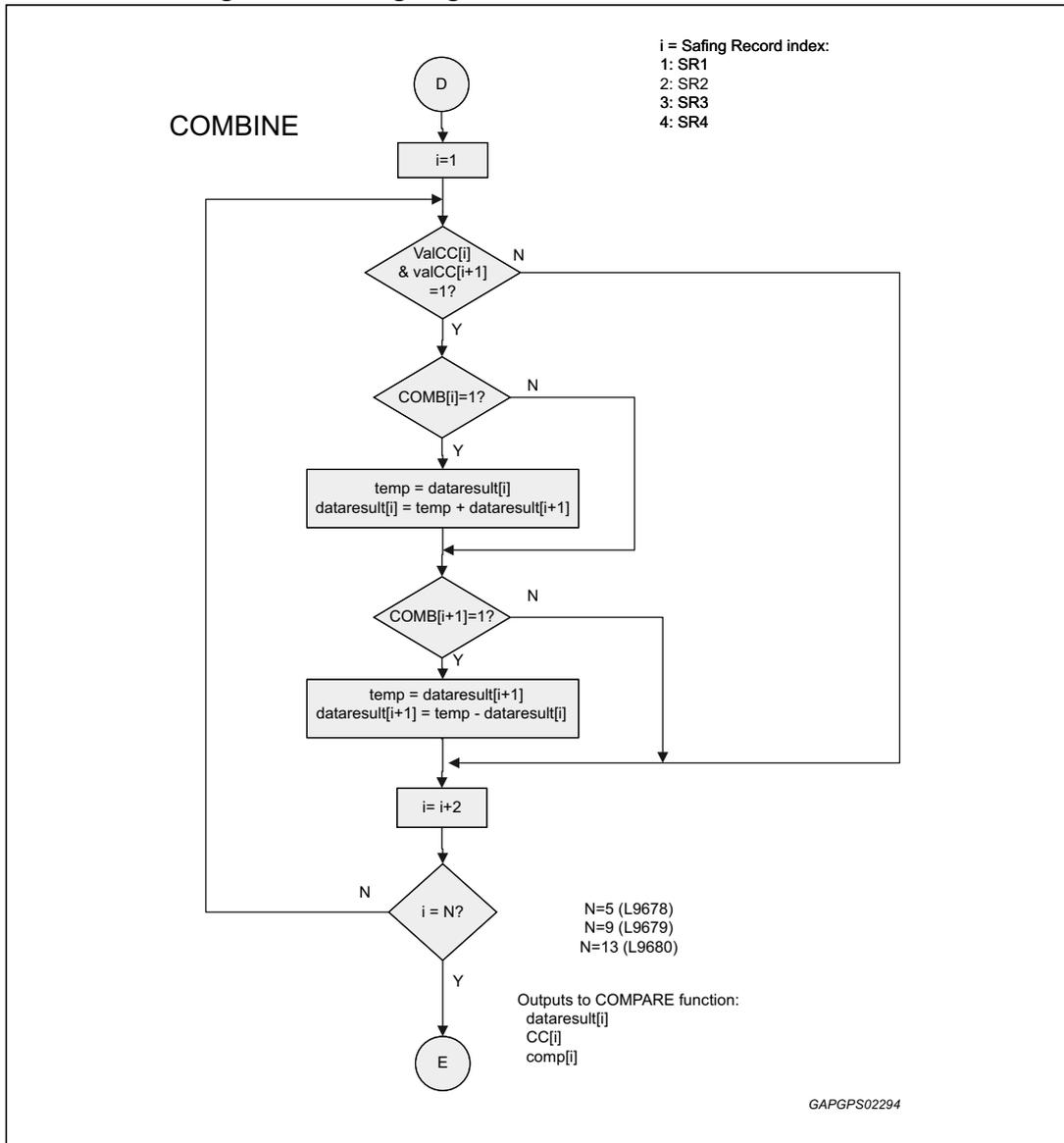
Figure 55. Safing engine threshold comparison
