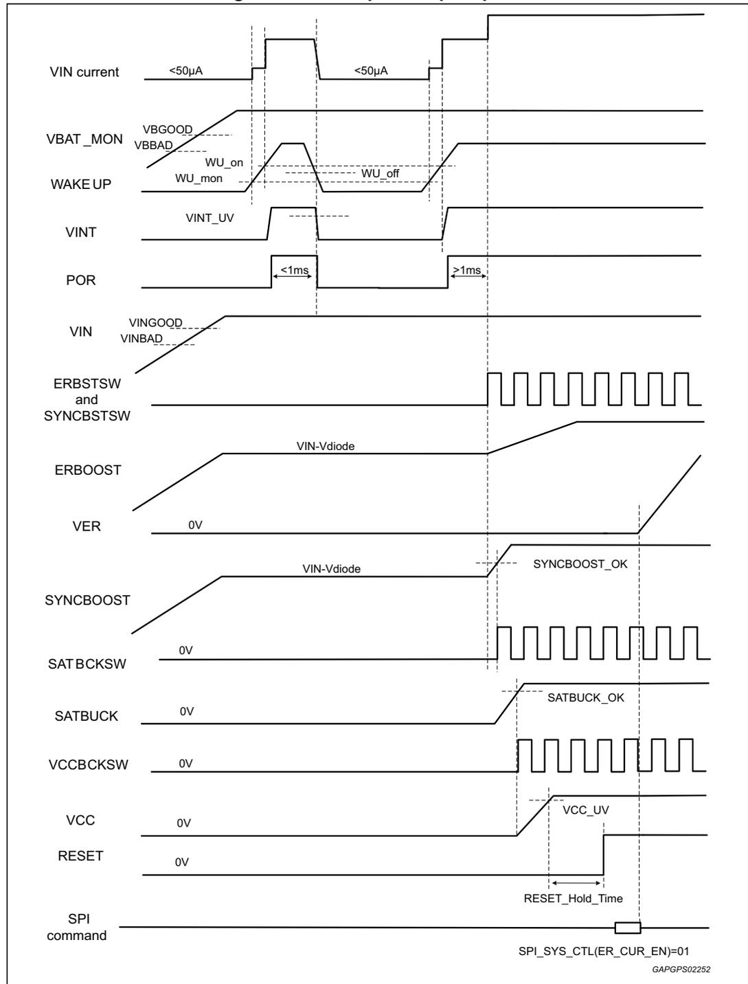
Figure 8. Normal power down sequence through Powermode Shutdown state - ER cap active discharge
