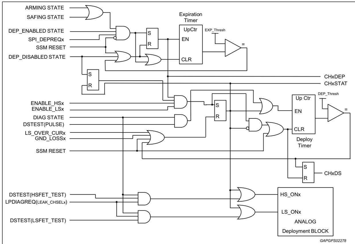
The high level block diagram for the deployment drivers is shown below:
