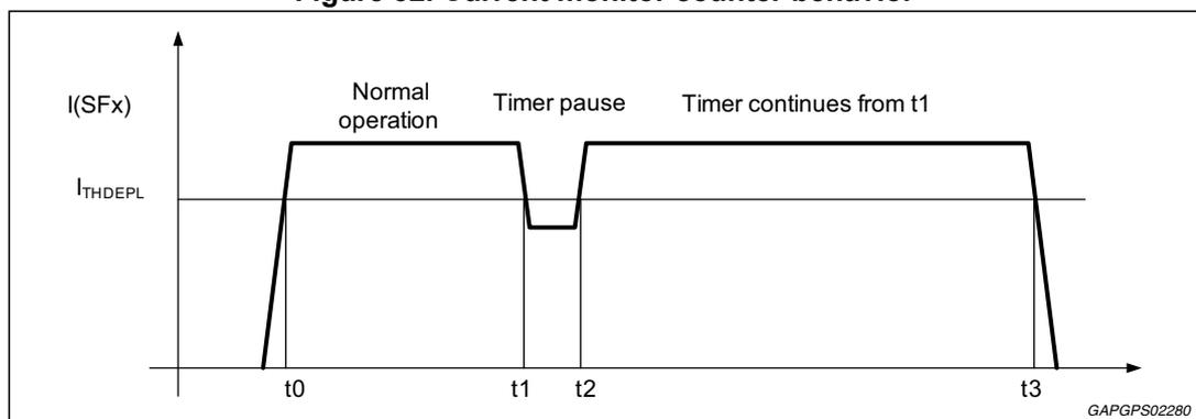
The deploy current counter is reset to \$0000 as soon as a toggle on DEP\_DISABLED is performed and a new DEPCOM command on the same channel is received.
