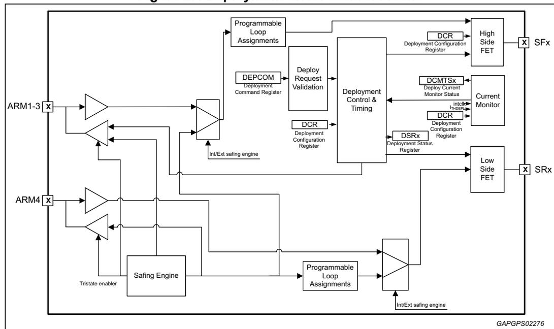
Figure 28. Deployment driver control logic - Enable signal
