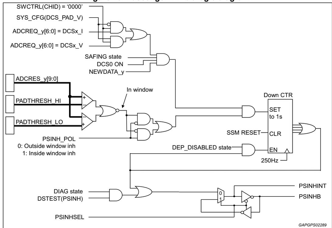
An upper and lower threshold is preprogrammed via SPI by writing the desired 10-bits values into the PADTHRESH\_HI and PADTHRESH\_LO registers during the Diag state. These thresholds define the measurement window where the passenger restraints are active. Any measurement outside this window will result in the assertion of the PSINHINT signal (as described below), thereby deactivating the squib loops identified in the PSINH mask. The PSINH mask is also preprogrammed during the Diag state.
