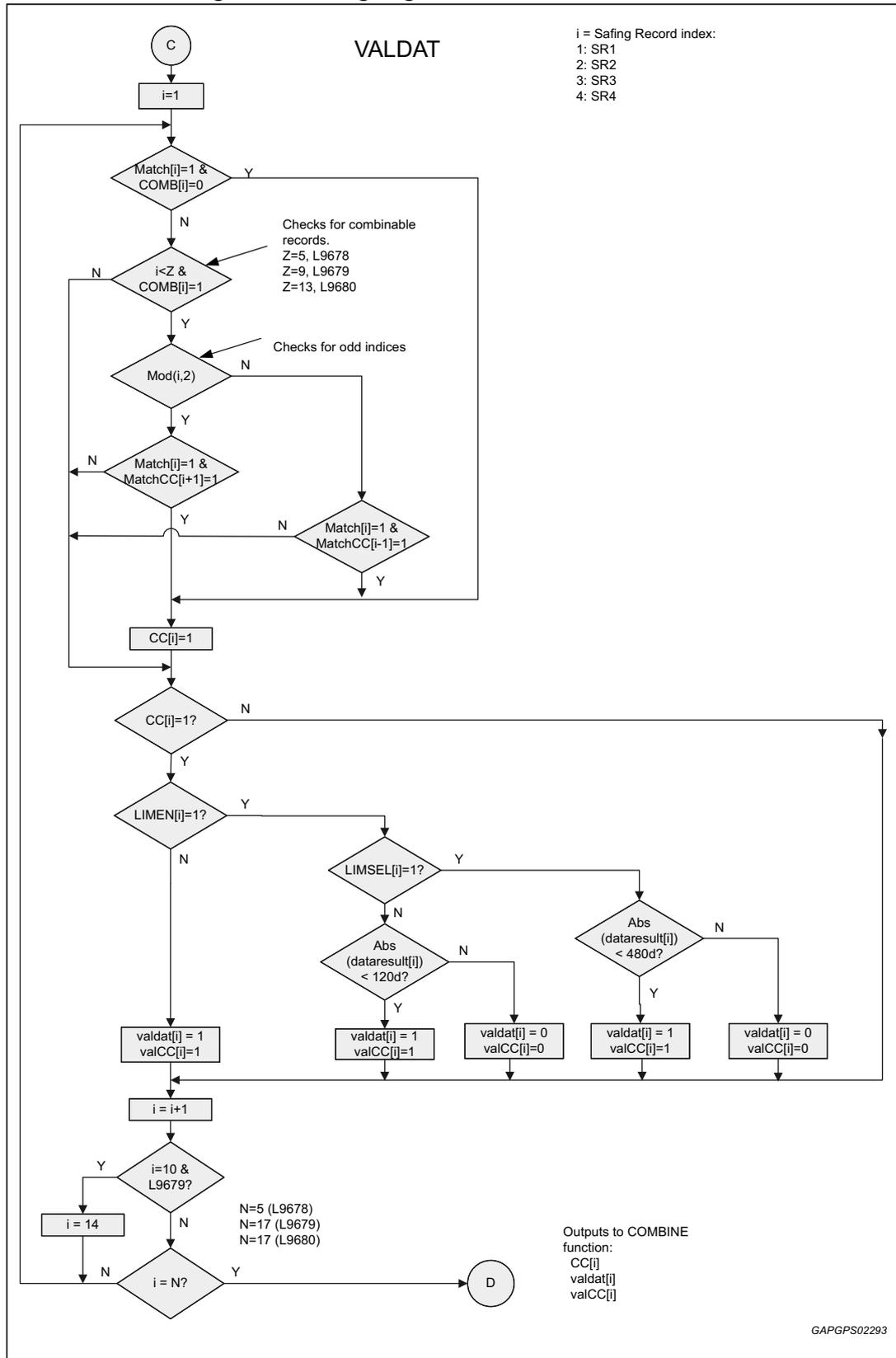
Figure 54. Safing engine - Combine function flow chart
