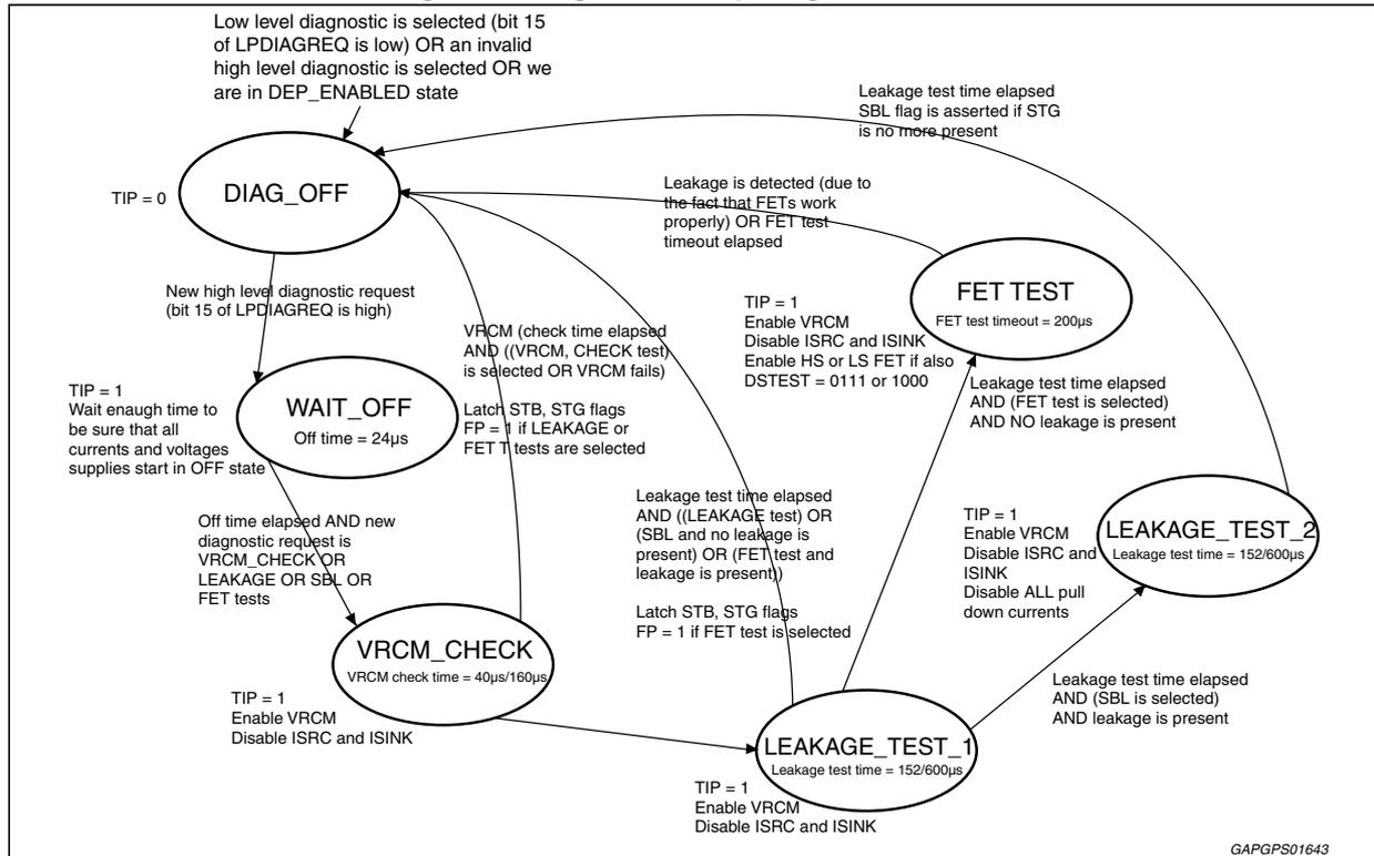
Figure 37. High level loop diagnostic flow2
