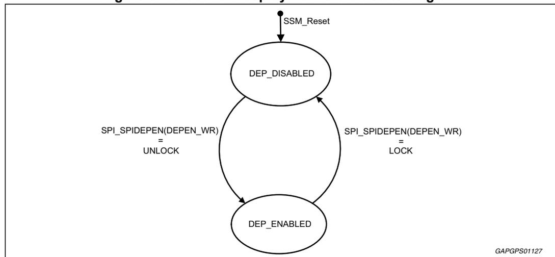
In case a multiple deployment request would be needed, i.e. deploying the same channel in sequence, a toggle on DEP\_DISABLED has to be performed and a new DEPCOM command on the same channel has to be sent.
