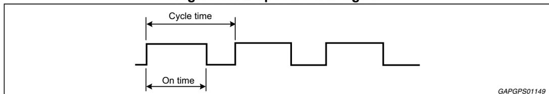
The disposal PWM signal cycle time and on time parameters can be found in the electrical parameters tables.
