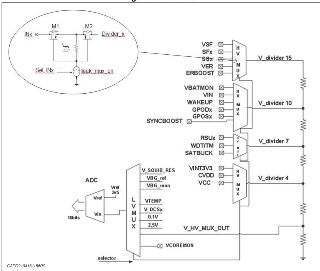
The diagnostics circuitry is activated by four SPI Diagnostics Control commands (DIAGCTRLx); each of them can address all the available nodes to be monitored, except for what mentioned in [Table 18](#).
