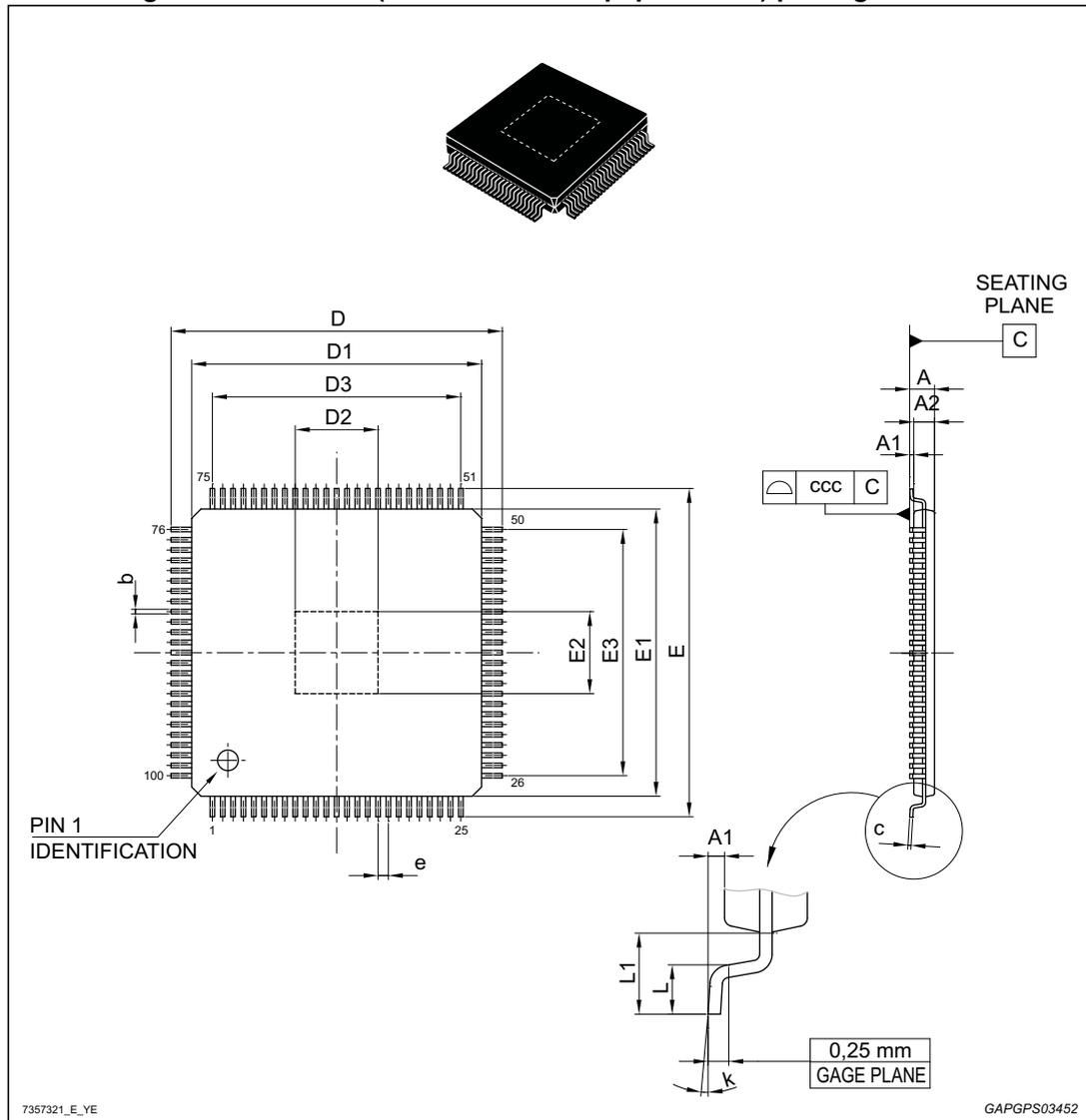
Table 74. TQFP100 (14x14x1.4 mm exp. pad down) package mechanical data
