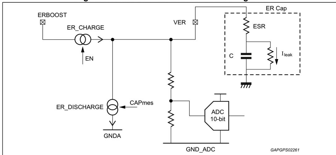
To obtain an accurate ER CAP measurement, the VER voltage conversion must be required when both current generators are off, namely no current flows through ER cap permits to avoid ESR error contribution.
