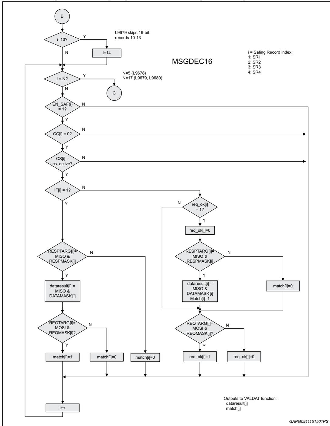
Figure 53. Safing engine - Validate data flow chart
