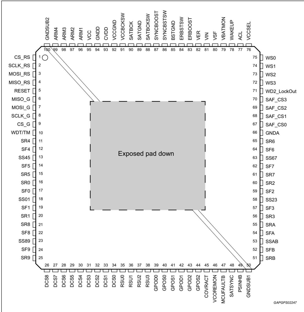
The exposed pad is electrically shorted to the substrate pins GNDSUB1 and GNDSUB2. These three connection nodes are to be kept shorted on the application.
