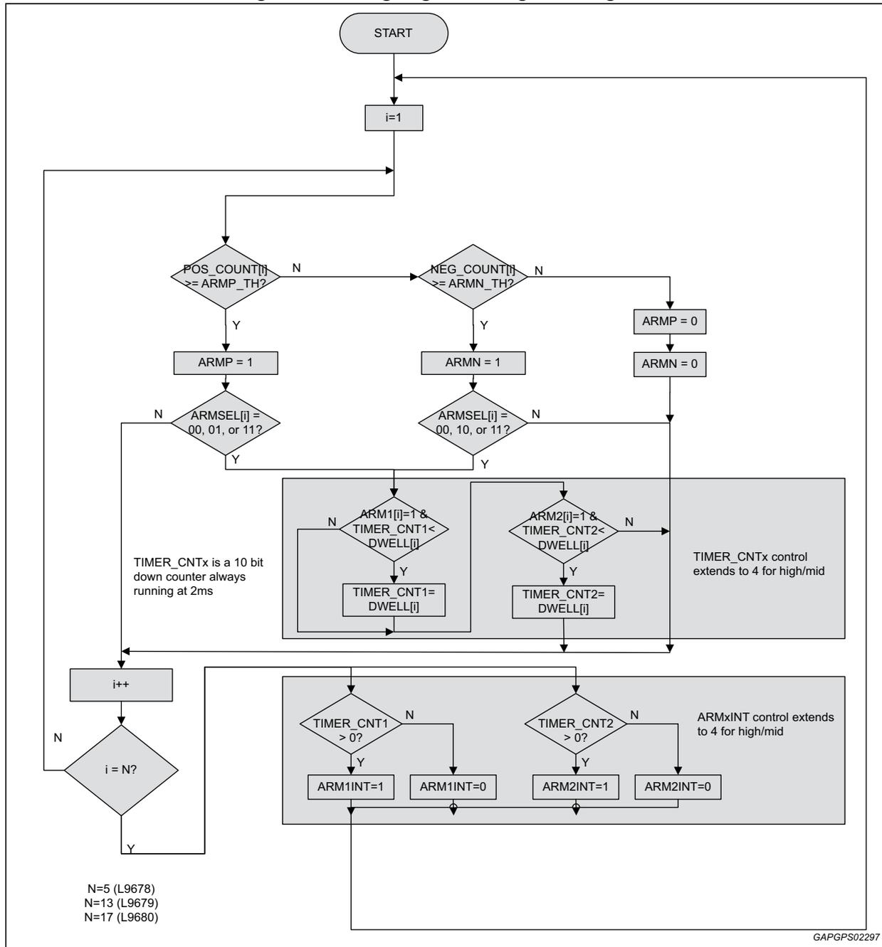
Figure 60. Safing engine diagnostic logic
