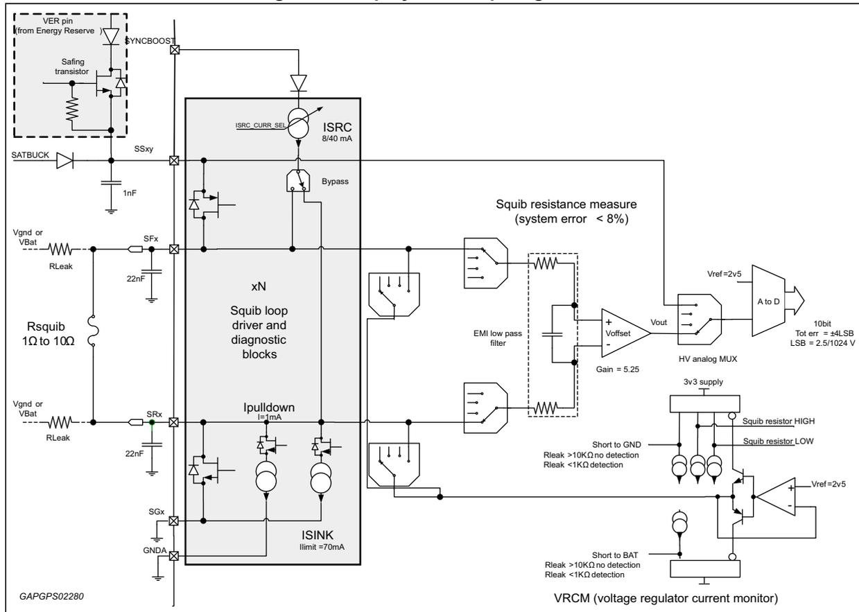
The leakage diagnostic includes short to battery, short to ground and shorts between loops. The test is applied to each SFx and SRx pin so shorts can be detected regardless of the resistance between the squib pins.
