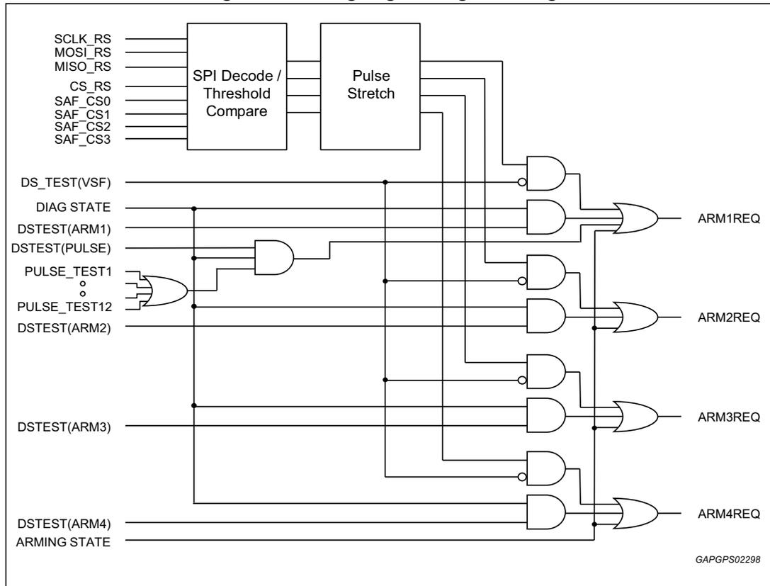
A configurable mask for each internal ARMxINT signal is available for all of the integrated deployment loops. The un-masked ARMxINT signal for each loop will enable the respective loop drivers.
