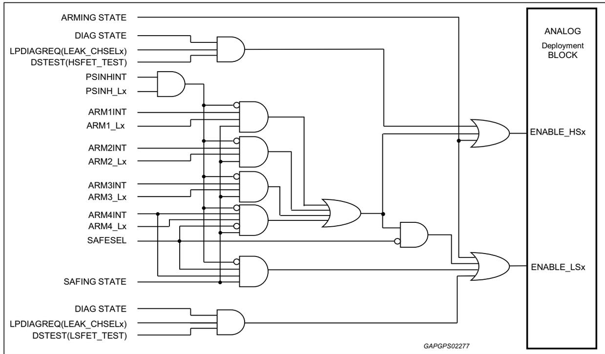
Figure 29. Deployment driver control logic - Turn-on signals
