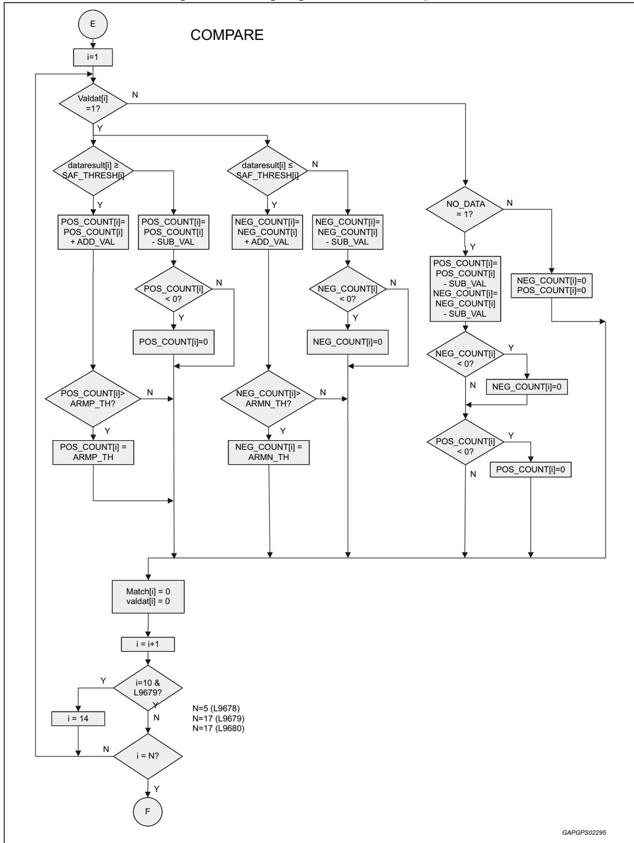
Figure 56. Safing engine - Compare complete
