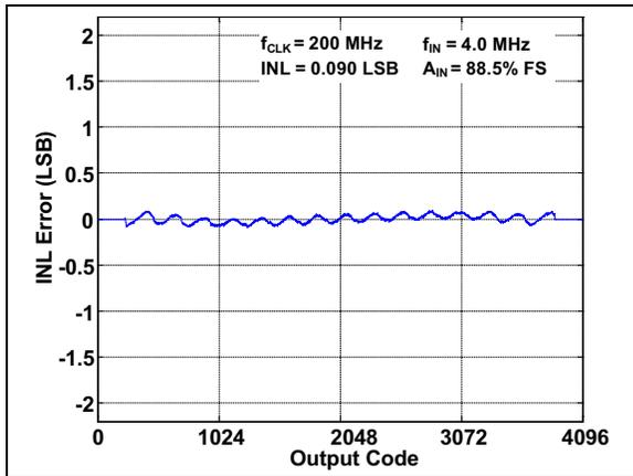
**FIGURE 3-41:** INL Error vs. Output Code:
