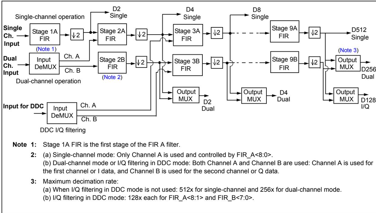
**FIGURE 4-16:** Simplified Block Diagram of Decimation Filters.
