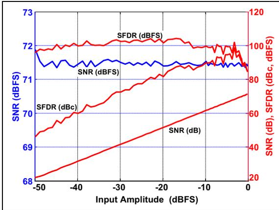
**FIGURE 3-24:** SNR/SFDR vs. Analog Input Amplitude:  $f_S = 200$  Msps,  $f_{IN} = 15$  MHz, High-Reference Mode (SENSE = AV<sub>DD12</sub>).
