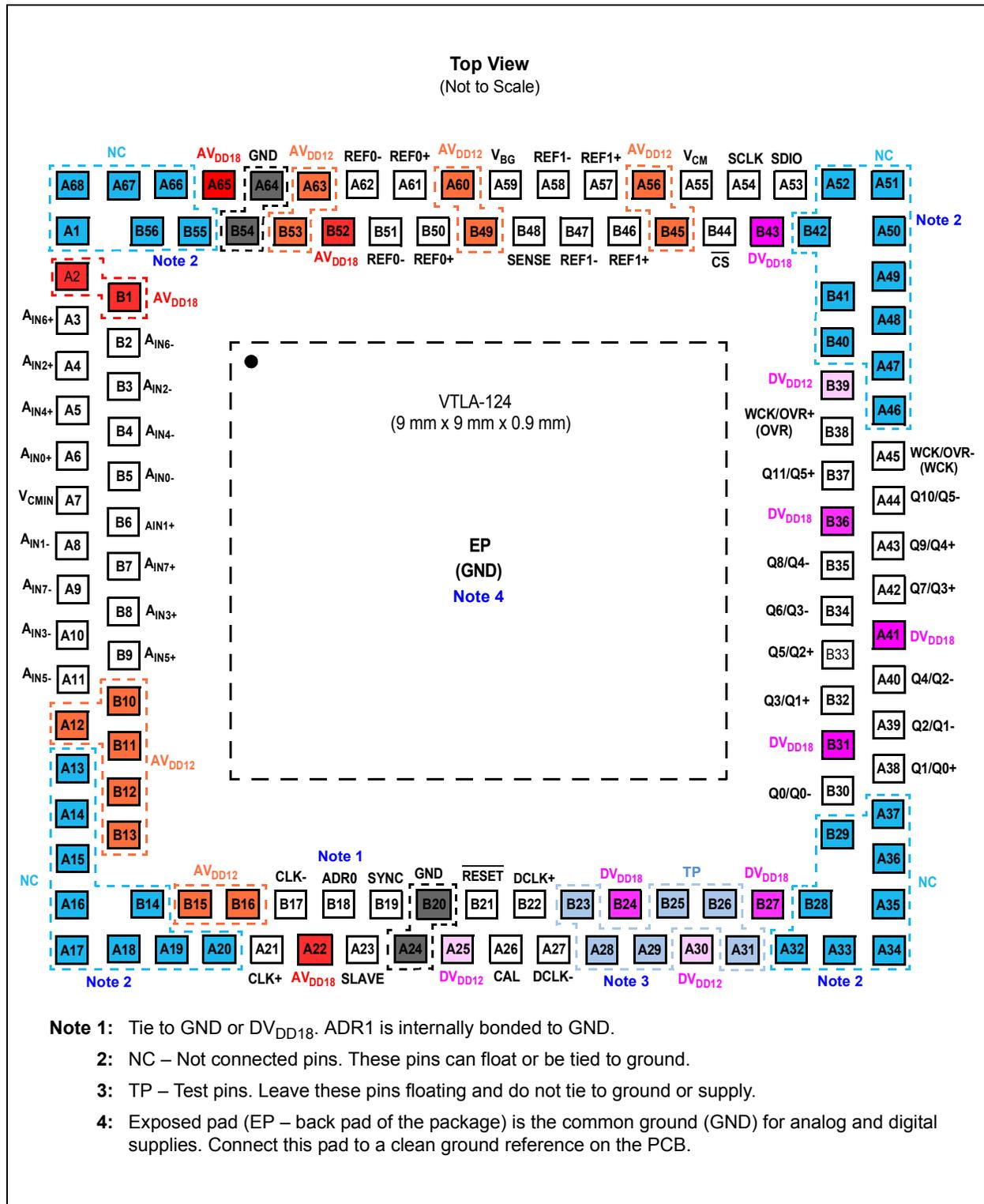
**FIGURE 1-1:** VTLA-124 Package. See Table 1-1 for the pin descriptions. Decoupling capacitors for reference pins and V<sub>BG</sub> are embedded in the package. Leave TP pins floating always.
