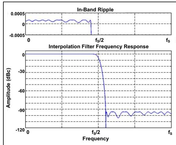
**FIGURE 4-13:** Response of the Dual-Channel Fractional Delay Recovery (1<sup>st</sup> Nyquist Band).  $f_s$  is the Sampling Frequency.
