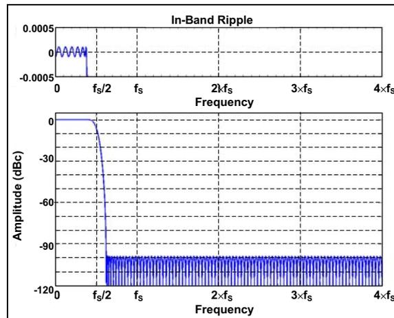
**FIGURE 4-14:** Response of the Octal-Channel Fractional Delay Recovery (1<sup>st</sup> Nyquist Band).  $f_s$  is the Sampling Frequency.
