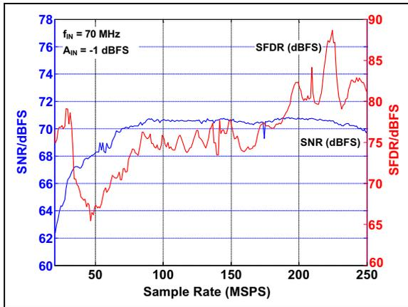
**FIGURE 3-30:** SNR/SFDR vs. Sample Rate (MSPs):  $f_{IN} = 70$  MHz.
