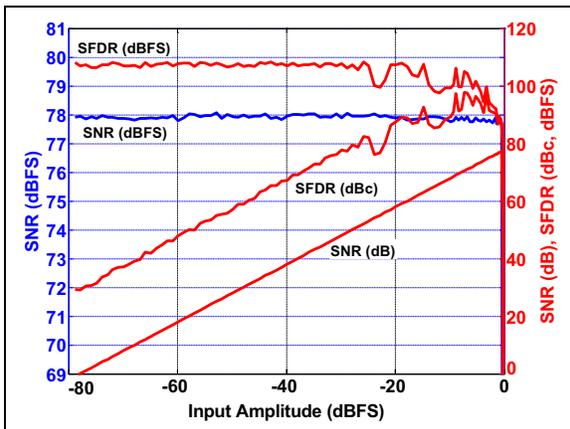
**FIGURE 3-26:** SNR/SFDR vs. Analog Input Amplitude:  $f_S = 200$  Msps,  $f_{IN} = 15$  MHz, High-Reference Mode (SENSE = AV<sub>DD12</sub>) with NSR enabled.  $A_{IN} \leq 0.8$  dBFS for NSR.
