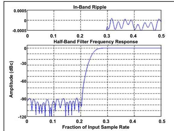
**FIGURE 4-20:** High-Pass (HP) Response of Half-Band Filter.
