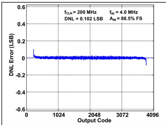
**FIGURE 3-42:** DNL Error vs. Output Code:
