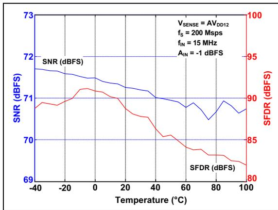
**FIGURE 3-36:** SNR/SFDR vs. Temperature:  $f_s = 200$  Mpsps,  $f_{IN} = 15$  MHz.
