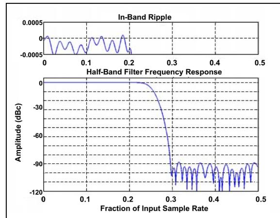
**FIGURE 4-21:** Low-Pass (LP) Response of Half-Band Filter.
