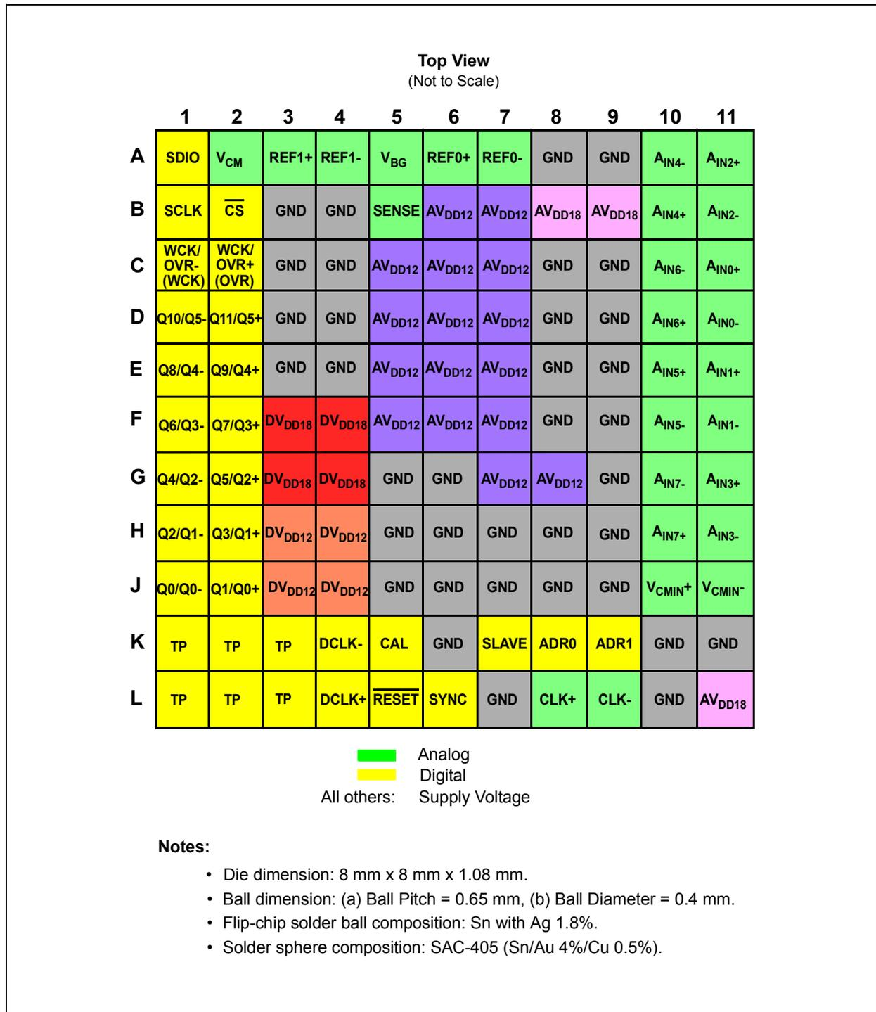
**FIGURE 1-2:** TFBGA-121 Package. See [Table 1-2](#) for the pin descriptions. Decoupling capacitors for reference pins and V<sub>BG</sub> are embedded in the package. Leave TP pins floating always.
