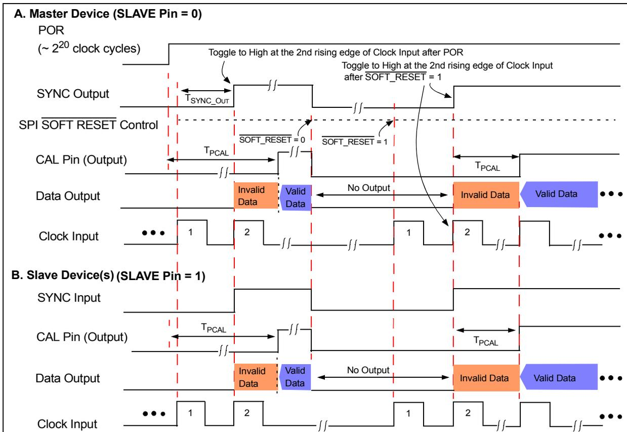
**FIGURE 2-9:** Sync Timing Diagram with  $\overline{SOFT\_RESET}$  Bit Setting.
