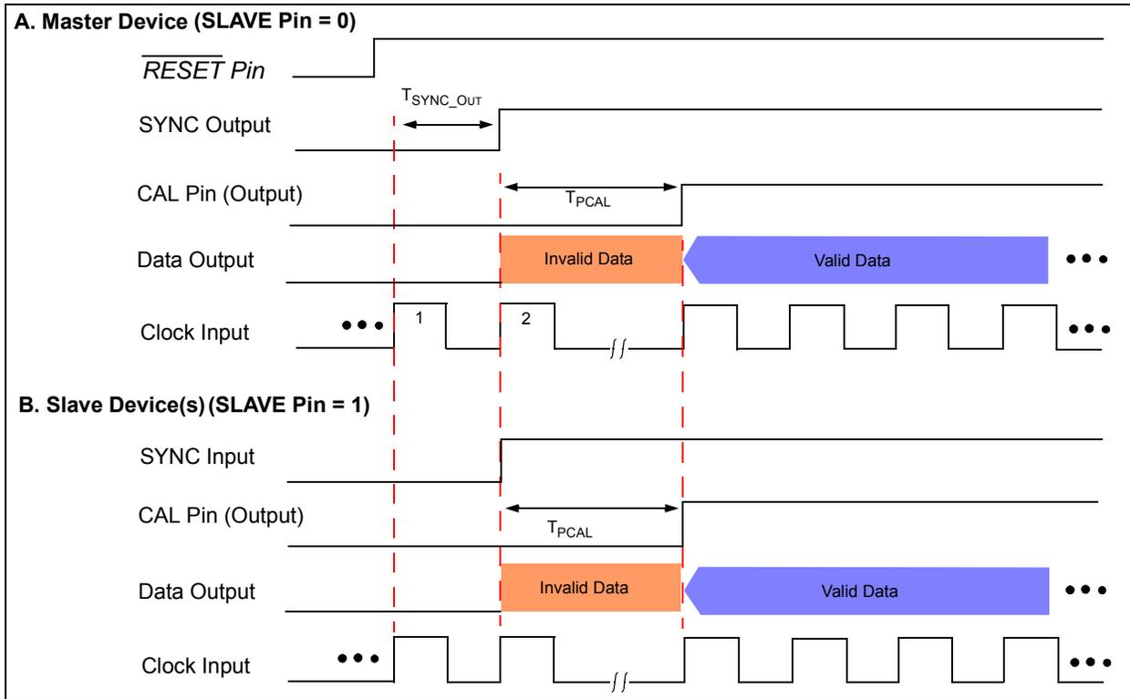
**FIGURE 2-8:** Sync Timing Diagram with  $\overline{RESET}$  Pin Operation.
