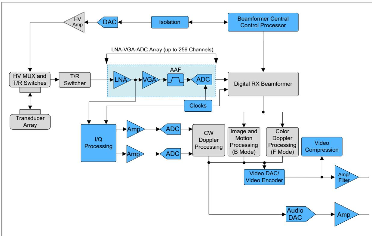
**FIGURE 4-23:** Example of Ultrasound System Building Block.
