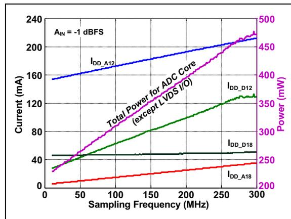
**FIGURE 3-46:** Power Consumption vs. Sampling Frequency (LVDS Mode).
