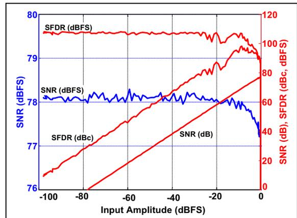
**FIGURE 3-29:** SNR/SFDR vs. Analog Input Amplitude:  $f_S = 200$  Msps,  $f_{IN} = 70$  MHz, High-Reference Mode (SENSE = AV<sub>DD12</sub>) with NSR enabled.  $A_{IN} \leq 0.8$  dBFS for NSR.
