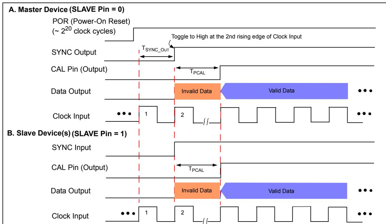
**FIGURE 2-7:** Sync Timing Diagram with Power-On Reset.
