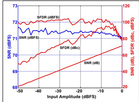
**FIGURE 3-27:** SNR/SFDR vs. Analog Input Amplitude:  $f_S = 200$  Msps,  $f_{IN} = 70$  MHz, High-Reference Mode (SENSE = AV<sub>DD12</sub>).
