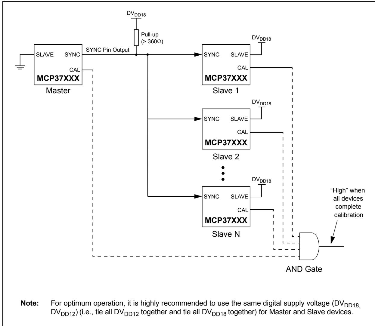
**FIGURE 4-28:** Synchronizing Multiple ADCs Using AutoSync Feature.
