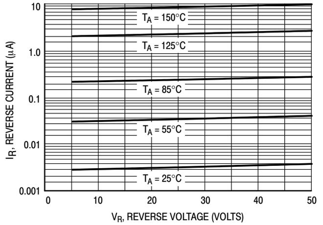
Figure 3. Leakage Current
