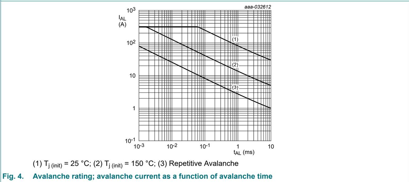
Fig. 4. Avalanche rating; avalanche current as a function of avalanche time
