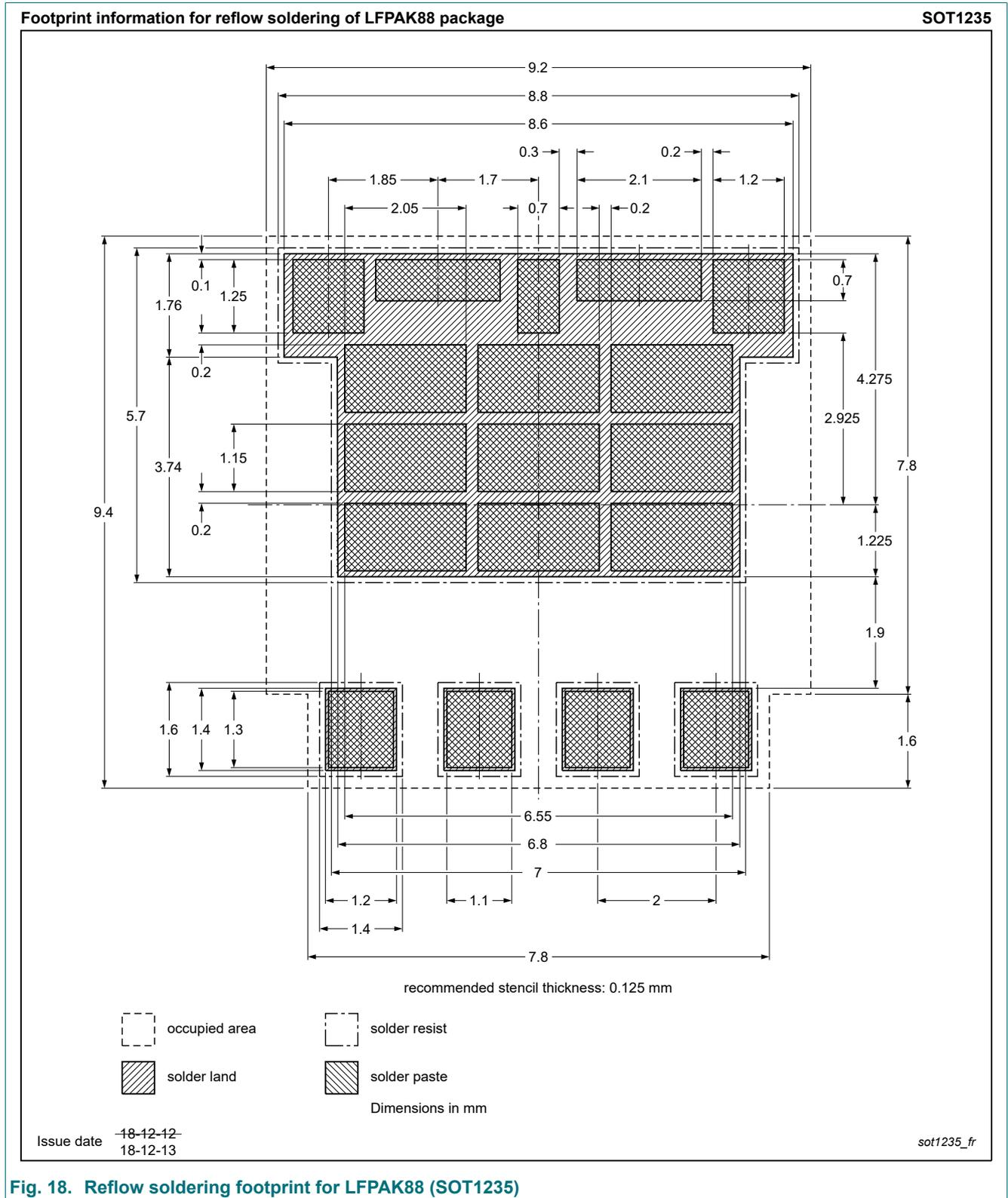
**Fig. 18. Reflow soldering footprint for LPAK88 (SOT1235)**
