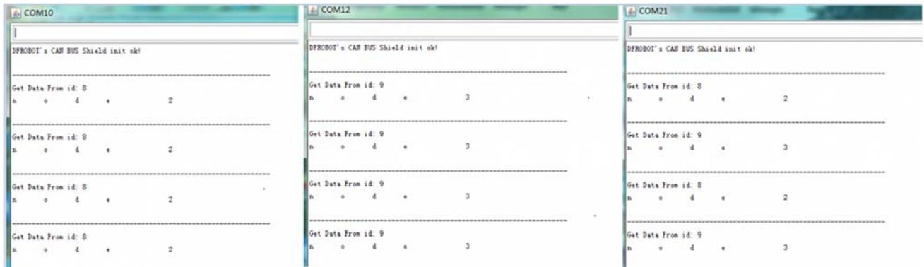
COM10 is running Node 3 code, which only receives the ID 0x08 data frame. COM12 is running Node 2 code, which only receives the ID 0x09 data frame. COM21 is running Node 1 code, which receives the ID 0x09 and 0x08 data frame.
