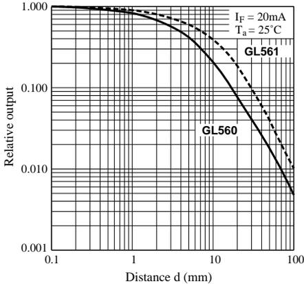
**Fig. 10 Relative Output vs. Distance (Detector : PD49PI)**
