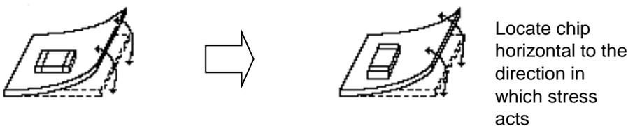
[Chip Mounting Close to Board Separation Point]
