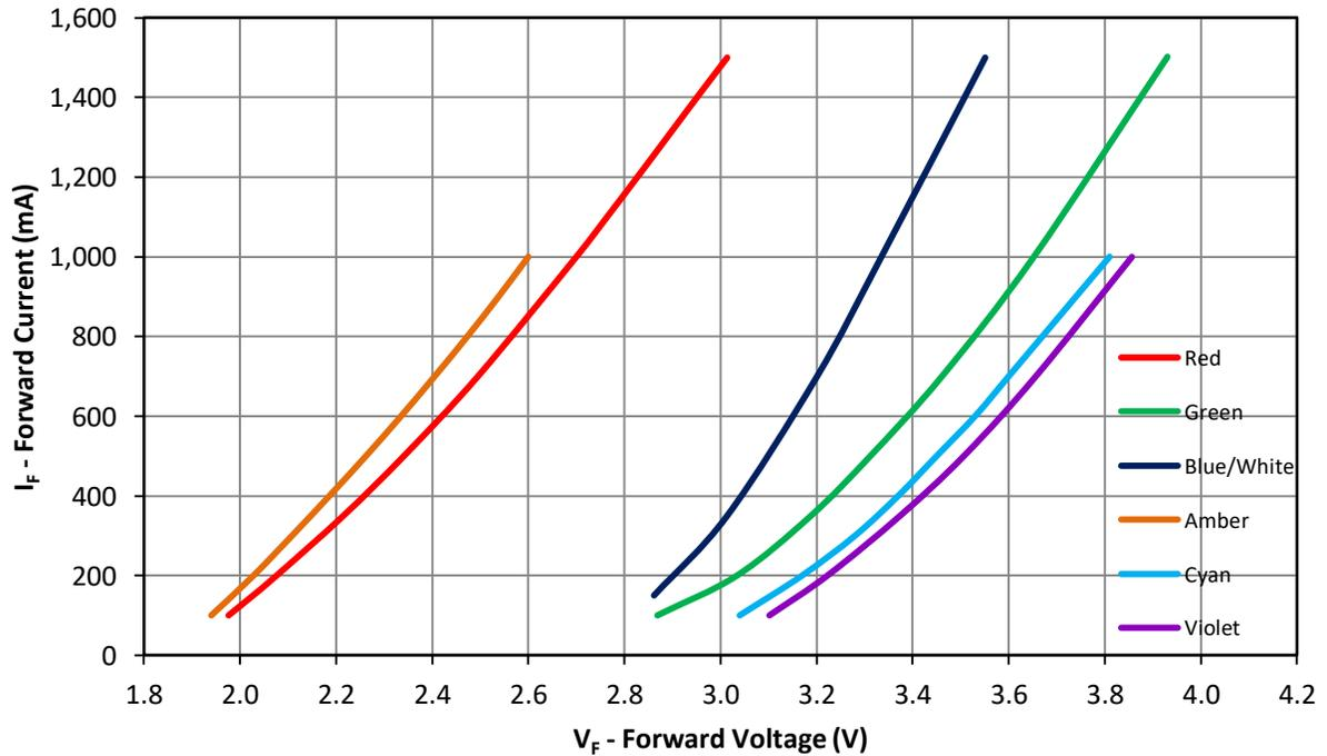
Figure 6: Typical forward current vs. forward voltage @ T<sub>c</sub> = 25°C
