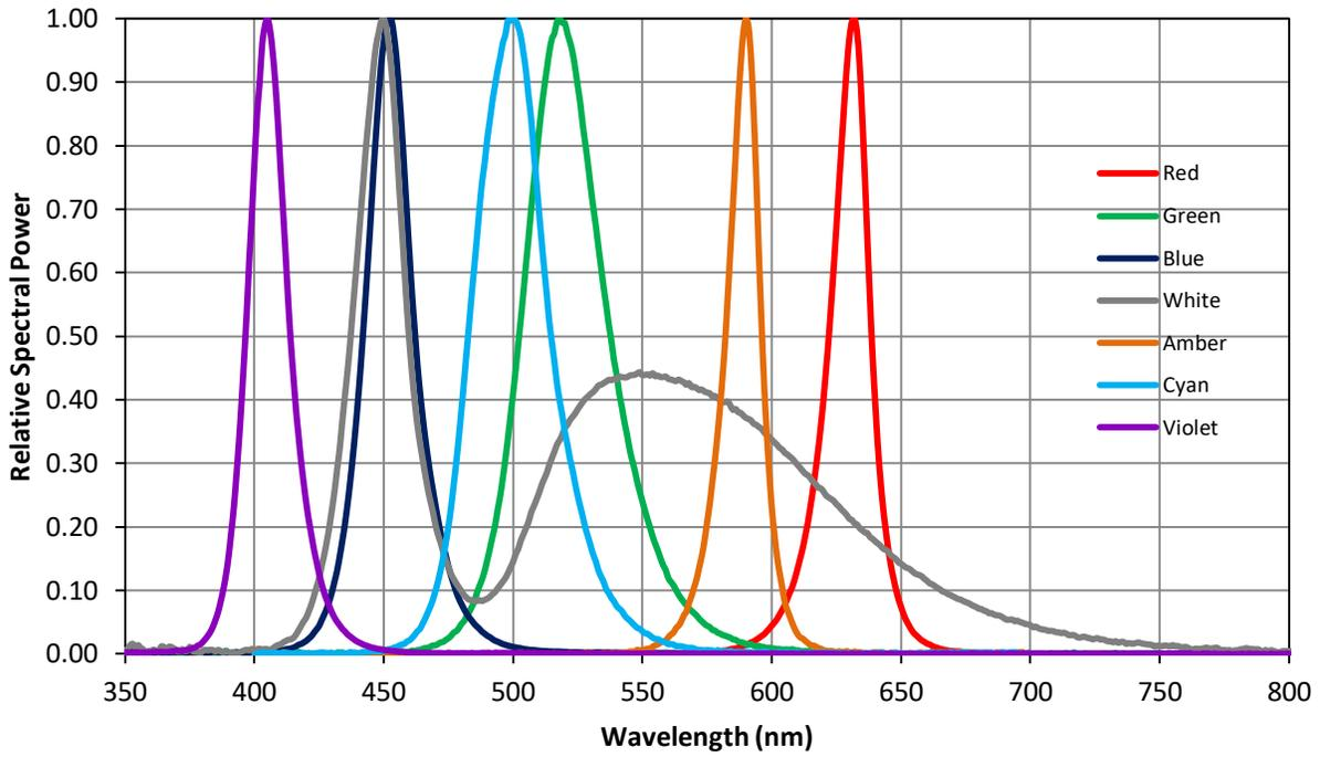
Figure 5: Typical relative spectral power vs. wavelength @ T<sub>c</sub> = 25°C.
