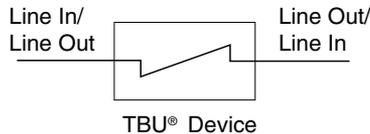
The TBU® high-speed protector placed in the system circuit will monitor the current with the MOSFET detection circuit triggering to provide an effective barrier behind which sensitive electronics will not be exposed to large voltages or currents during surge events up to the device's specified maximum limits. The TBU® device is provided in a surface mount DFN package and meets industry standard requirements such as RoHS and Pb Free solder reflow profiles.
