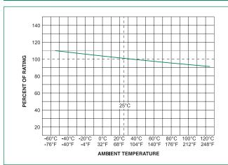
1. Re-rating depicted in this curve is in addition to the standard derating of 25% for continuous operation.
