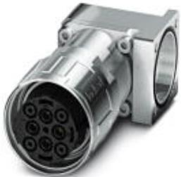
Device connector, front mounting with knurled nut, angled fixed, SPEEDCON locking, M40, Number of positions: 2+3+PE, Type of contact: Socket, Crimp connection, Axial O-ring, 4x Ø4,2, Shielded: Yes, Flange dimensions: 40 mm x 40 mm
