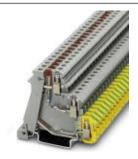
Sensor/actuator terminal block, Cross section: 0.2 mm² - 4 mm², AWG: 24 - 12, Connection type: Screw connection, Width: 6.2 mm, Color: gray, Mounting type: NS 35/7,5, NS 35/15
