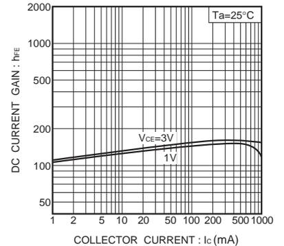
Fig.3 DC current gain vs. collector current ( I )
