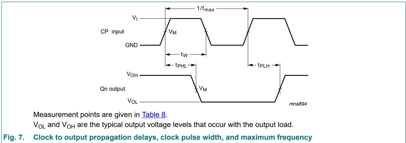
9-bit D-type flip-flop with 5 V tolerant inputs/outputs; positive edge-trigger; 3-state
