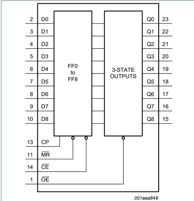
Fig. 1. Functional diagram
