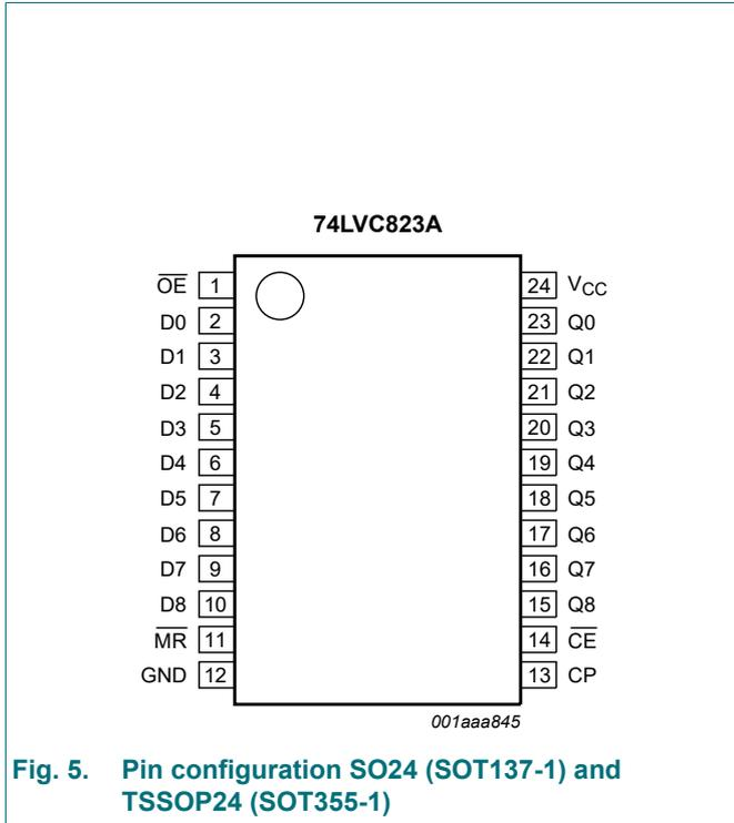
Fig. 5. Pin configuration SO24 (SOT137-1) and TSSOP24 (SOT355-1)
