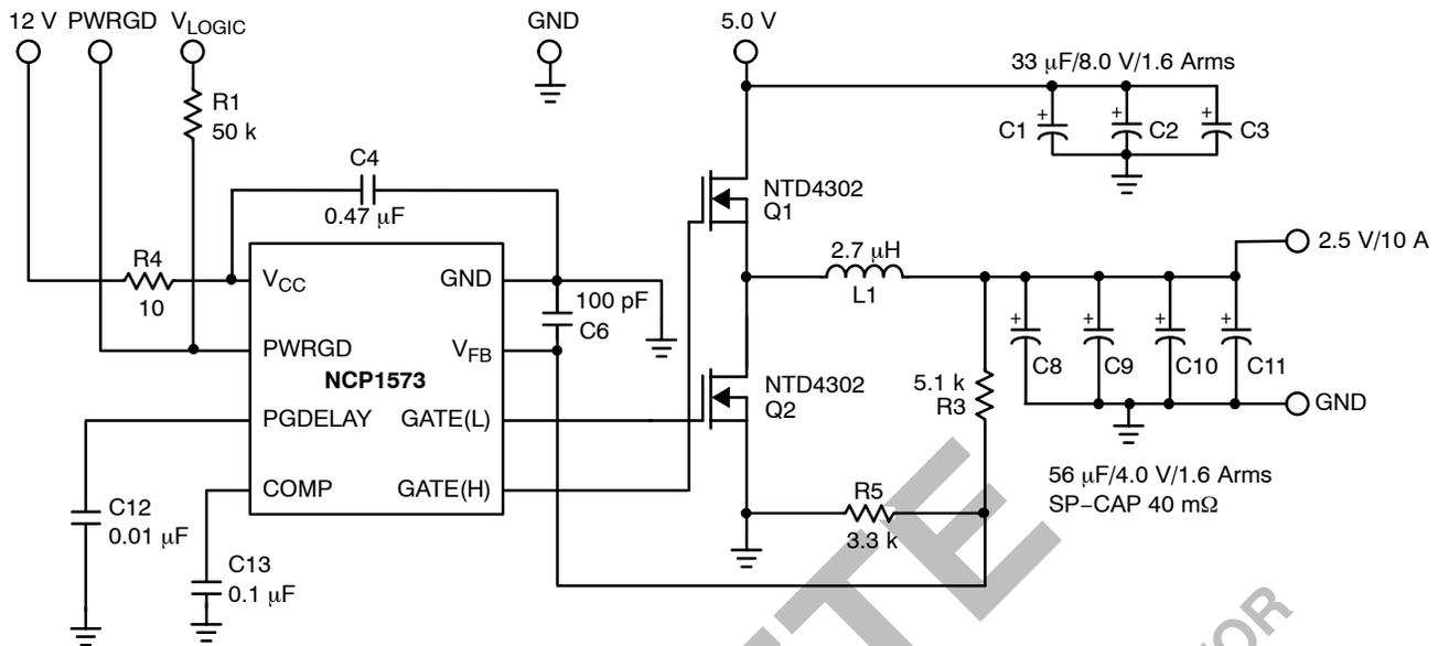
Figure 1. Applications Circuit
