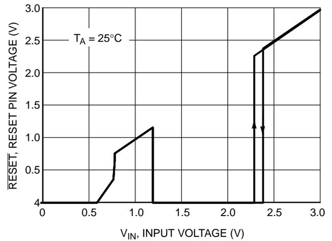
Figure 18. RESET Pin Voltage vs. Input Voltage
