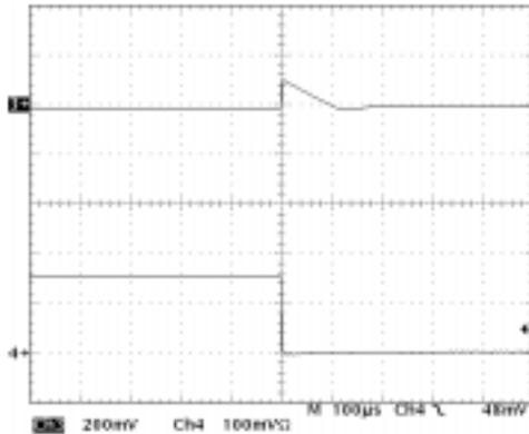
$I_{OUT} = 150 \text{ mA to } 1 \text{ mA}, V_{IN} = 3.3 \text{ V}, C_{IN} = 1 \mu\text{F}$
