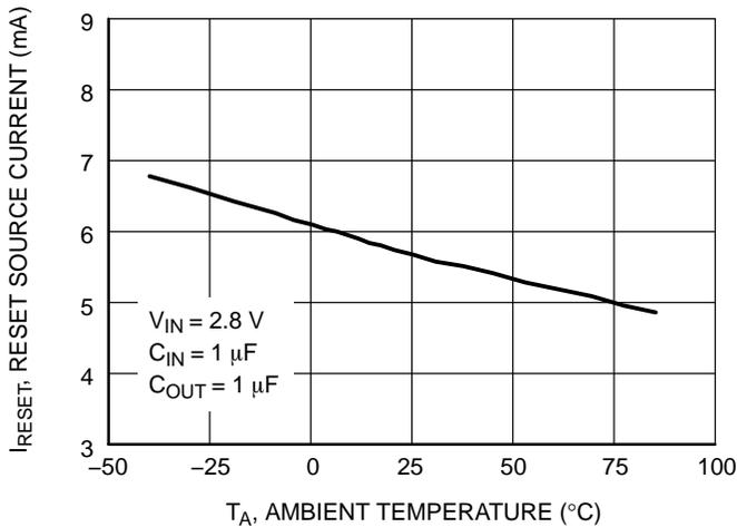
**Figure 13. RESET Pin P-Channel Source Current vs. Temperature**
