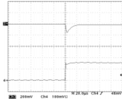
$I_{OUT} = 1 \text{ mA to } 150 \text{ mA}, V_{IN} = 3.3 \text{ V}, C_{IN} = 1 \mu\text{F}$
