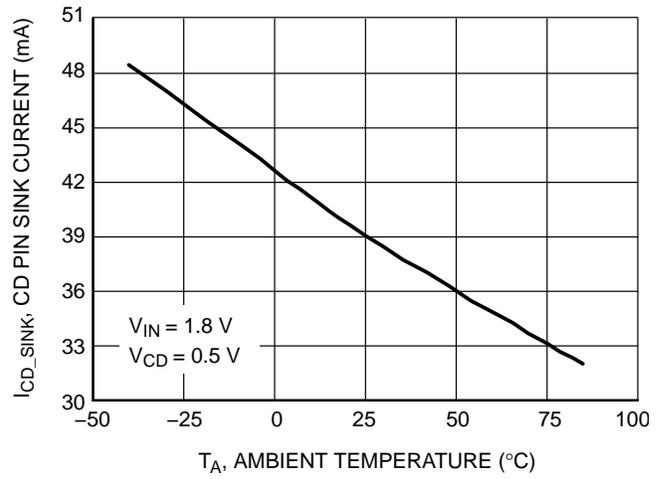
Figure 16. CD Pin Sink Current vs. Temperature
