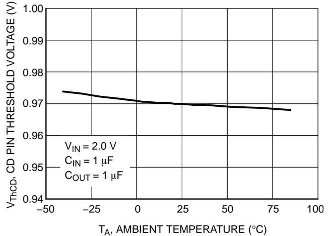
**Figure 14. CD Delay Pin Threshold Voltage vs. Temperature**
