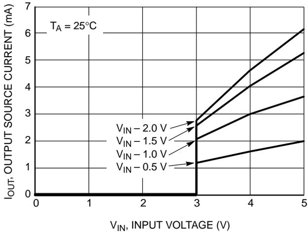
**Figure 21. Reset Output Source Current vs. Input Voltage**
