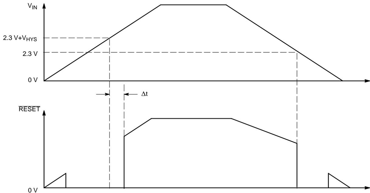
Figure 24. Timing Diagram
