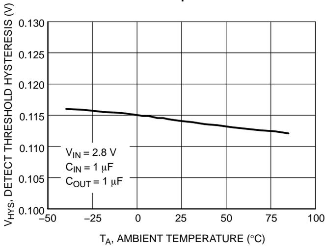
**Figure 11. Detector Threshold Hysteresis Voltage vs. Temperature**
