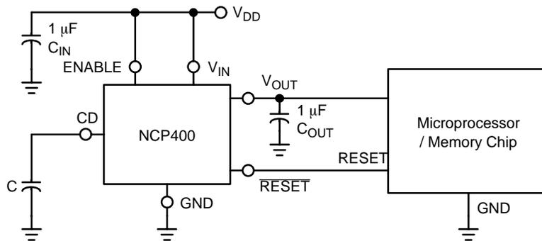
$$\text{DelayTime : } (\Delta t) = \frac{(C \times 0.97 \text{ V})}{1.56 \mu\text{A}}$$
