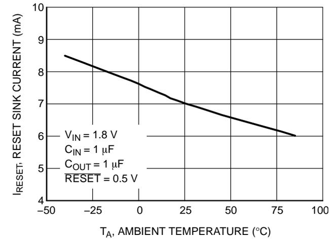
**Figure 12. RESET Pin N-Channel Sink Current vs. Temperature**
