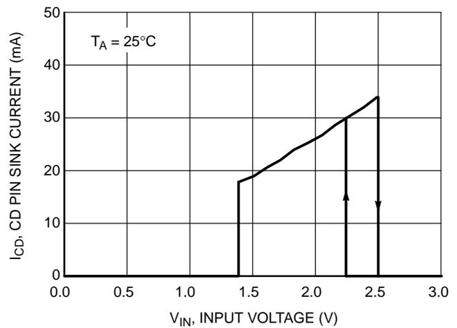
Figure 20. CD Pin Sink Current vs. Input Voltage
