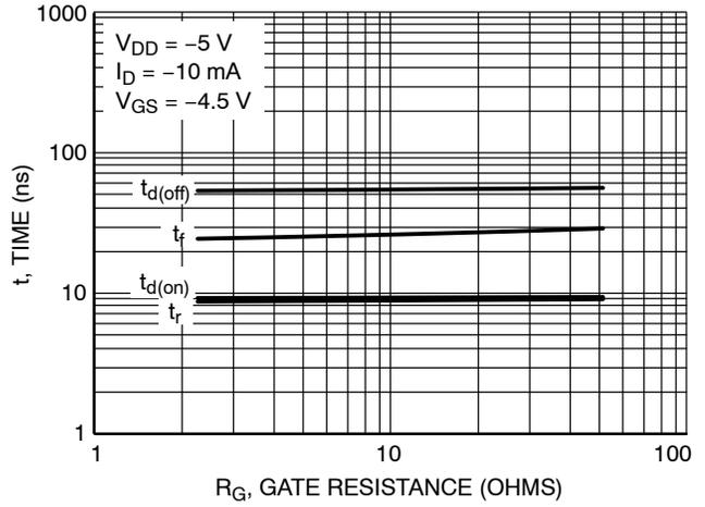
Figure 8. Resistive Switching Time Variation vs. Gate Resistance
