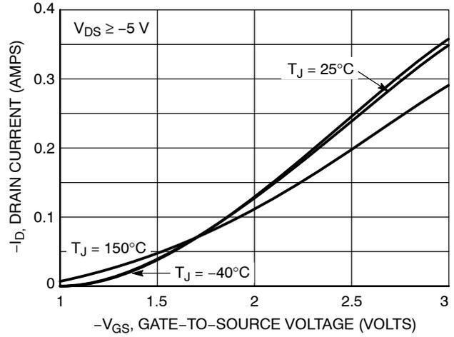
Figure 2. Transfer Characteristics
