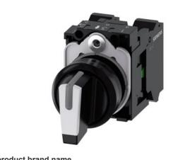
Selector switch, illuminable, 22 mm, round, plastic, white, selector switch, short, 3 switch positions I>O<II, momentary contact type, 10:30h/12h/13:30h, with holder, 1 NO, 1 NO, spring-type terminal, with laser labeling, upper case and lower case, always upper case at beginning of line
