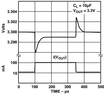
Figure 14. Load Transient for 10 mA to 100 mA Pulse
