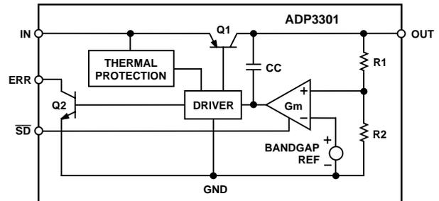
The ADP3301 operates with a wide input voltage range from 3 V to 12 V and delivers a load current in excess of 100 mA. It features an error flag that signals when the device is about to lose regulation or when the short circuit or thermal overload protection is activated. Other features include shutdown and optional noise reduction capabilities. The ADP330x anyCAP™\* LDO family offers a wide range of output voltages and output current levels from 50 mA to 200 mA:
