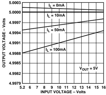
Figure 2. Line Regulation: Output Voltage vs. Input Voltage
