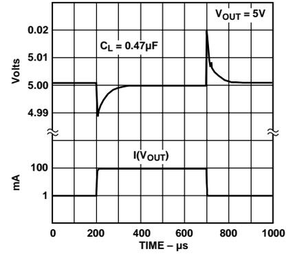
Figure 13. Load Transient for 1 mA to 100 mA Pulse
