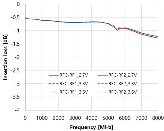
**Figure 5 Insertion Loss vs. Temp (RFC - RFx)**
