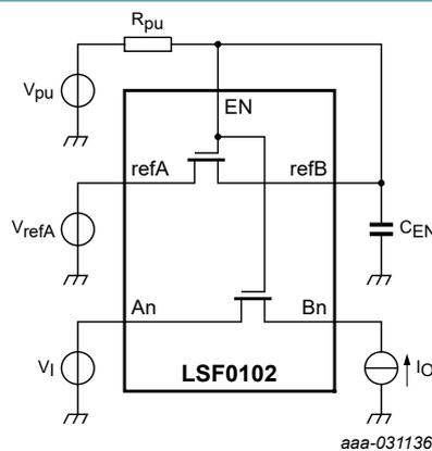
R<sub>pu</sub> = 200 kΩ; C<sub>EN</sub> = 100 nF (The An and Bn pins may be exchanged.)
