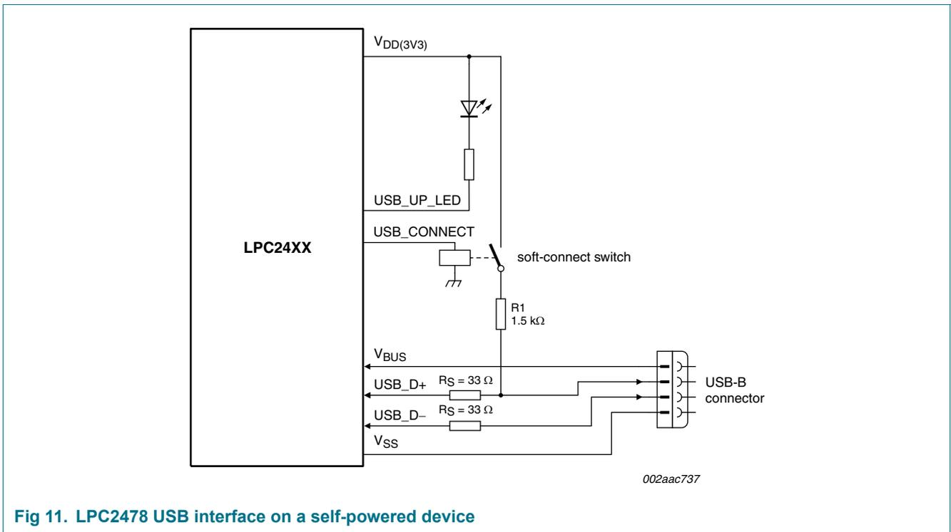
Fig 11. LPC2478 USB interface on a self-powered device
