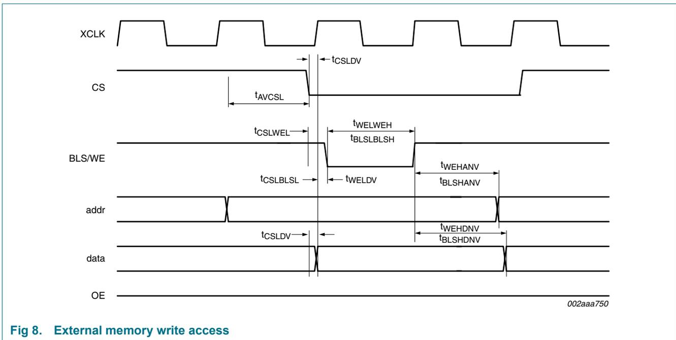
Fig 8. External memory write access
