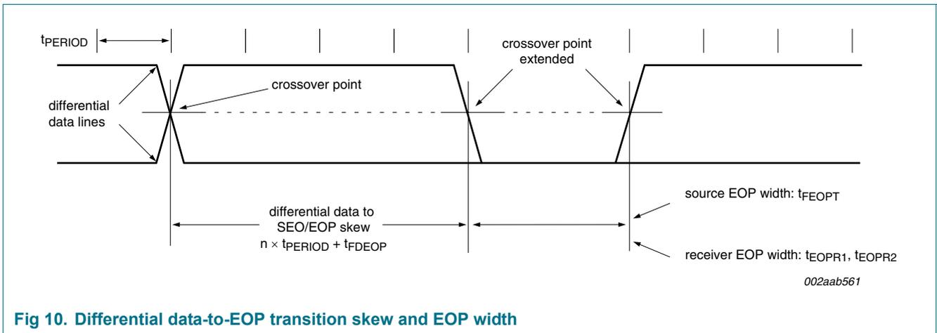
Fig 10. Differential data-to-EOP transition skew and EOP width
