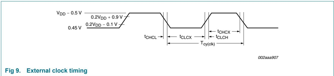
Fig 9. External clock timing
