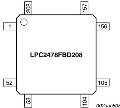
Fig 2. LPC2478 pinning LQFP208 package
