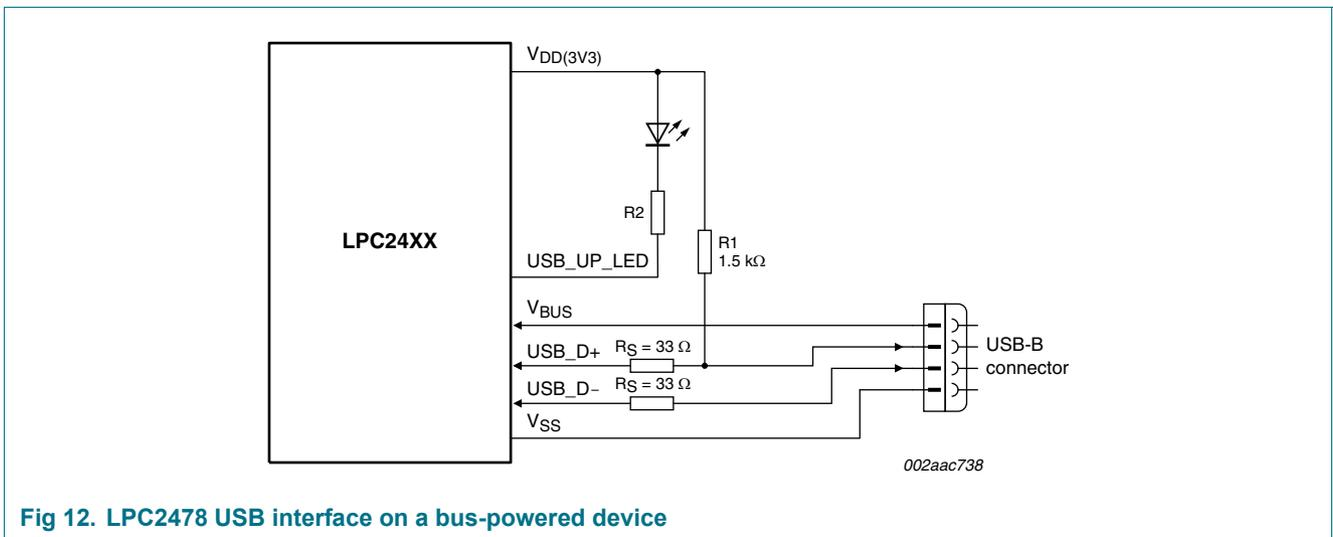
Fig 12. LPC2478 USB interface on a bus-powered device
