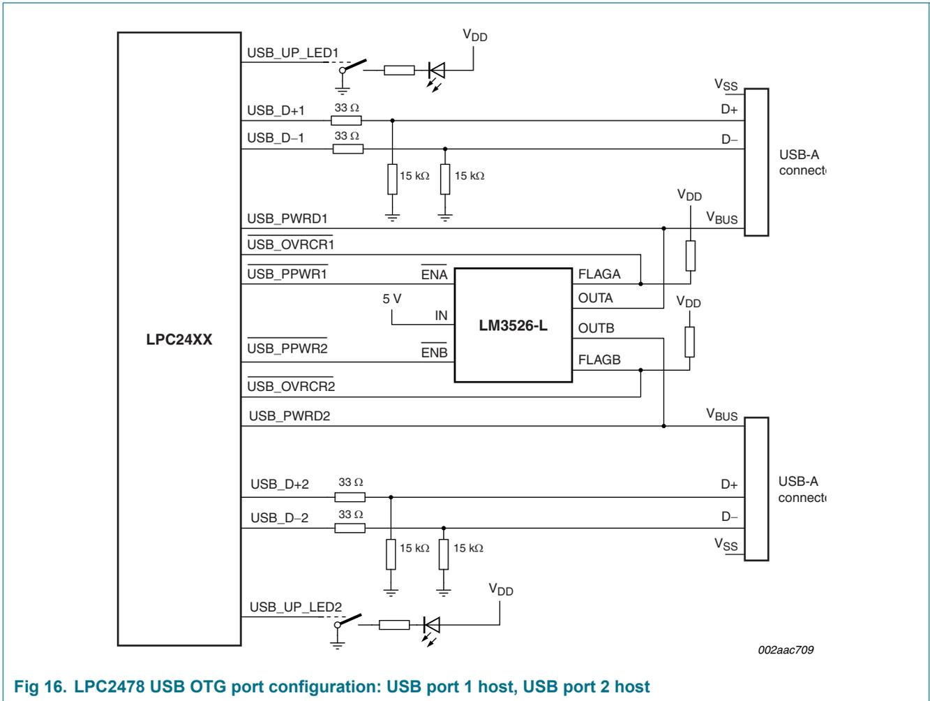
Fig 16. LPC2478 USB OTG port configuration: USB port 1 host, USB port 2 host
