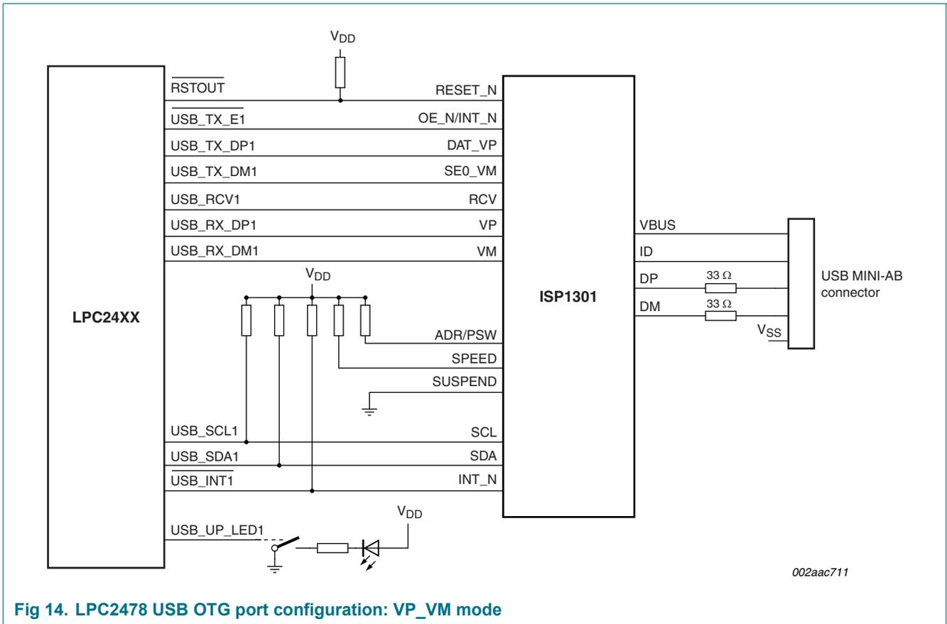
Fig 14. LPC2478 USB OTG port configuration: VP\_VM mode
