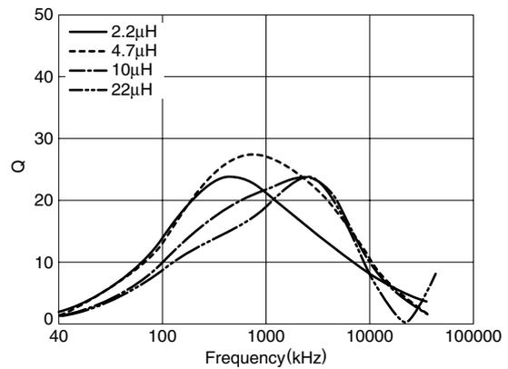
• Test equipment: YHP4194A IMPEDANCE/GAIN-PHASE ANALYZER(10kHz to 40MHz)
