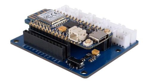
This Shield can break out the processor pins of Wio Lite (for instance, it is SAM D21 for Wio Lite W600) into the form of header and Grove connectors. There are 4 Grove digital connectors and 4 Grove analog connectors, a Grove UART port, and a Grove I2C port. As you can see, a switch is there for input power selection. If you use USB to power your Wio Lite board, then select the 5V mode, and if you use the lipo battery, please select the 3.3V.
