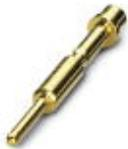
Crimp contact, turned, Single contact, Contact diameter: 1 mm, Crimp range: 0.06 mm<sup>2</sup>...0.25 mm<sup>2</sup>
