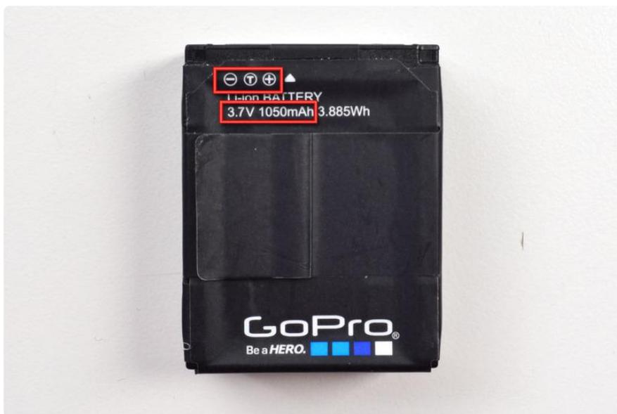
You can see its a 3.7V 1000mAh battery. That means we can charge it at 500mA max rate if we wish.
