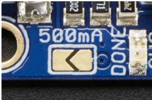
Melt some solder onto the jumper to close it and set the new charge rate
