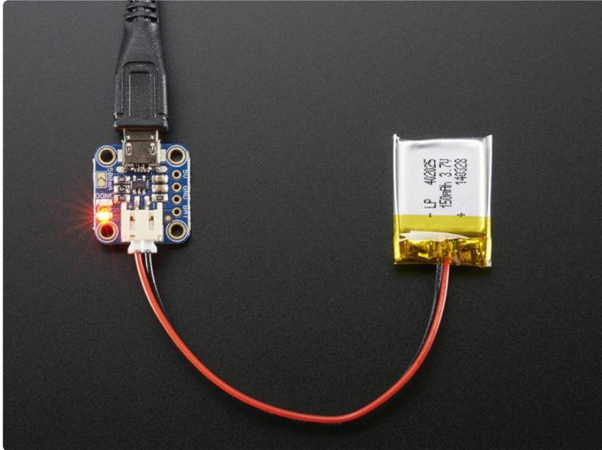
You can plug in either the battery first or the USB port first. We provide a JST jack since the large number of batteries we carry come with a JST PH connector or cable
