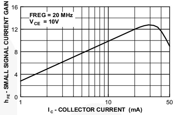
Figure 8. Small Signal Current Gain vs. Collector Current
