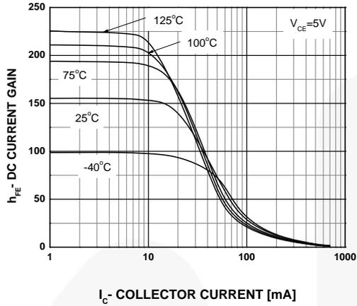
Figure 1. Typical Pulsed Current Gain vs. Collector Current
