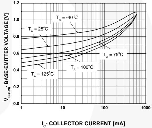
Figure 4. Base-Emitter On Voltage vs. Collector Current
