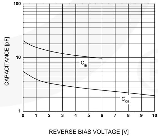
Figure 6. Input and Output Capacitance vs. Reverse Voltage
