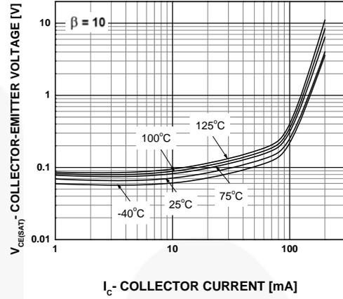
Figure 2. Collector-Emitter Saturation Voltage vs. Collector Current
