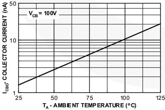
Figure 5. Collector Cut-Off Current vs. Ambient Temperature
