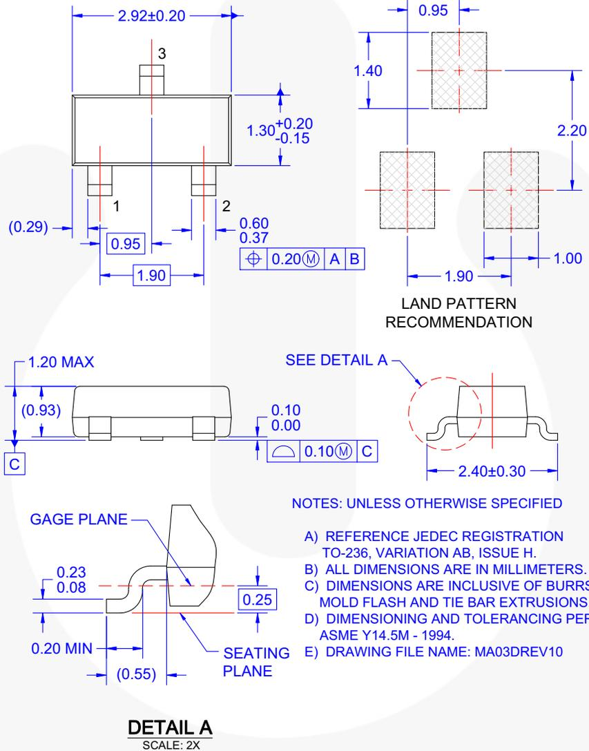
Figure 12. 3-LEAD, SOT23, JEDEC TO-236, LOW PROFILE (ACTIVE)
