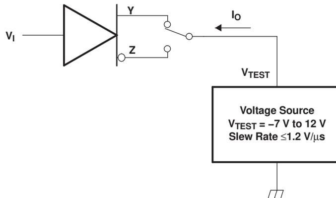
Figure 13. Test Circuit, Short-Circuit Output Current
