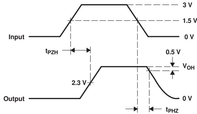
PRR = 1 MHz, 50% duty cycle,  $t_r < 6$  ns,  $t_f < 6$  ns,  $Z_O = 50 \Omega$
