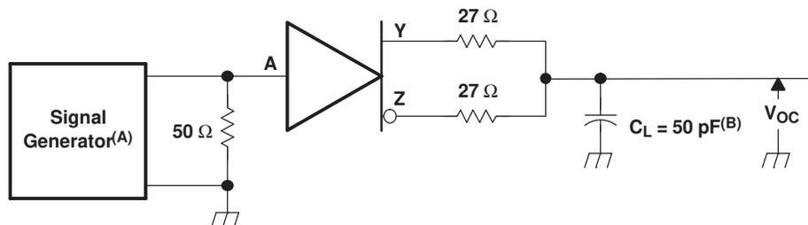
PRR = 1 MHz, 50% duty cycle,  $t_r < 6$  ns,  $t_f < 6$  ns,  $Z_O = 50 \Omega$
