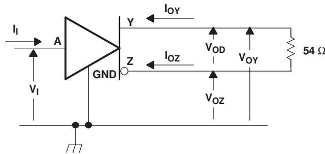
Figure 7. Test Circuit,  $V_{OD}$  Without Common-Mode Loading
