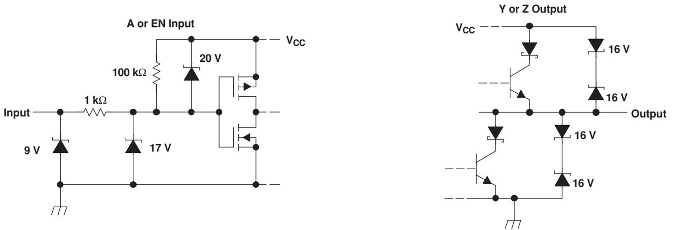
Figure 15. Equivalent Input and Output Schematic Diagrams
