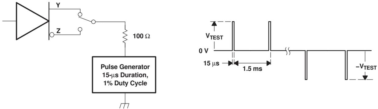
Figure 14. Test Circuit Waveform, Transient Overvoltage Test
