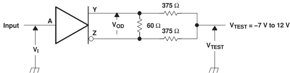
Figure 8. Test Circuit,  $V_{OD}$  With Common-Mode Loading
