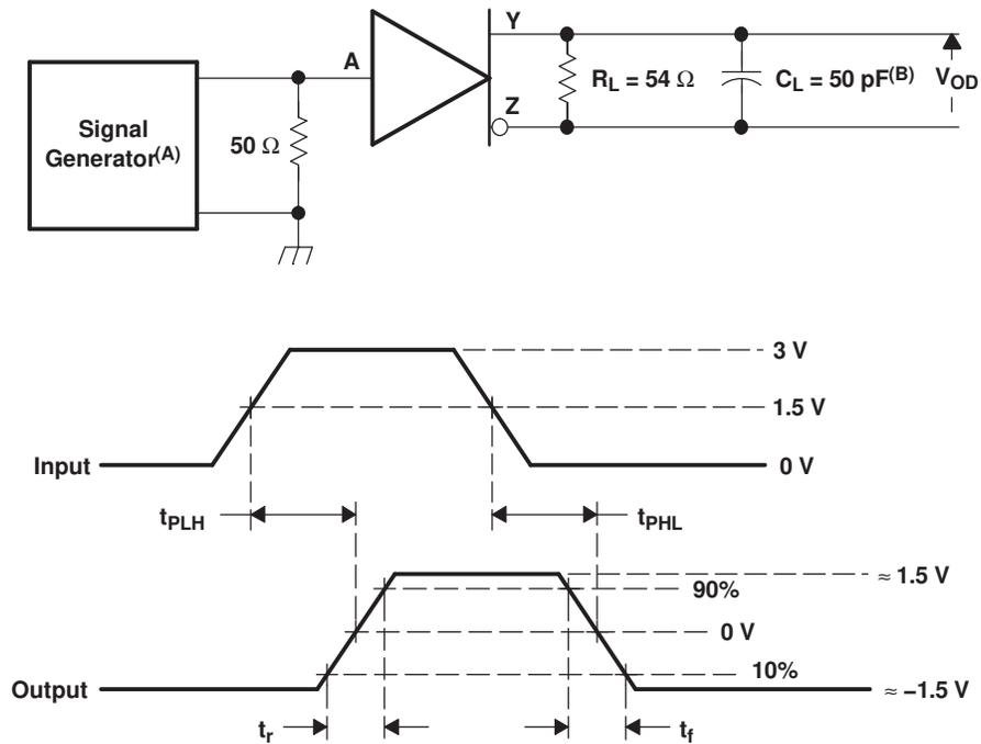
PRR = 1 MHz, 50% duty cycle,  $t_r < 6$  ns,  $t_f < 6$  ns,  $Z_0 = 50 \Omega$
