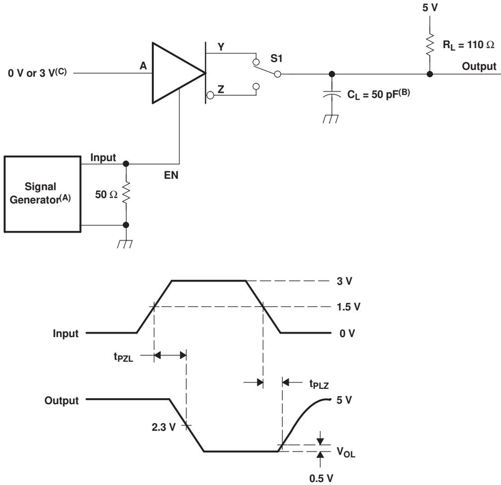
PRR = 1 MHz, 50% duty cycle,  $t_r < 6$  ns,  $t_f < 6$  ns,  $Z_O = 50 \Omega$
