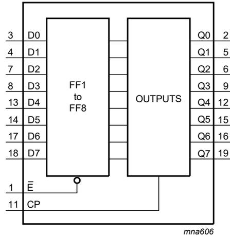
Fig. 1. Functional diagram
