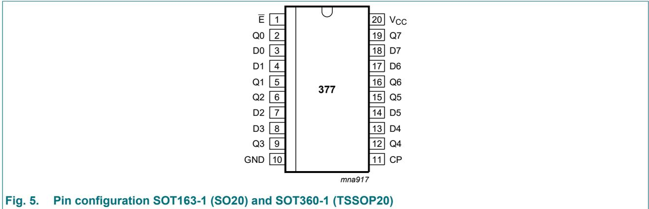
Fig. 5. Pin configuration SOT163-1 (SO20) and SOT360-1 (TSSOP20)
