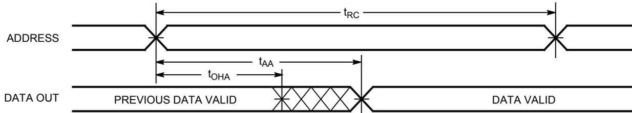
Figure 5. Read Cycle No. 2:  $\overline{OE}$  Controlled [19, 20]
