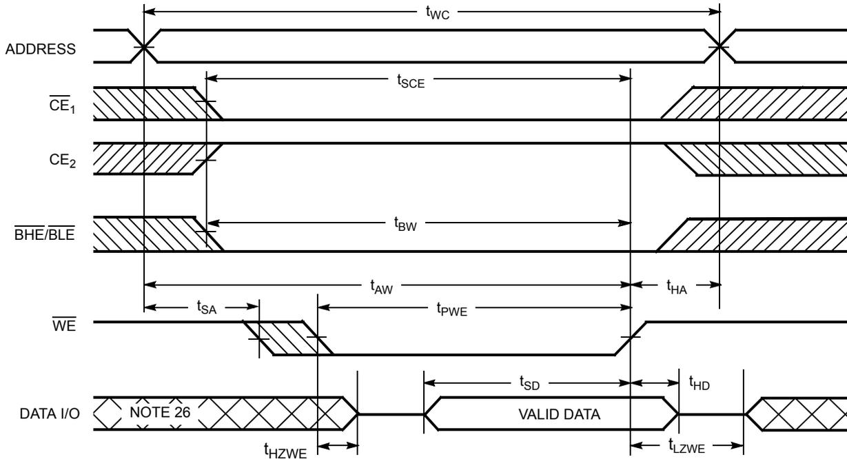
Figure 9. Write Cycle 4:  $\overline{BHE}/\overline{BLE}$  Controlled,  $\overline{OE}$  LOW [25]
