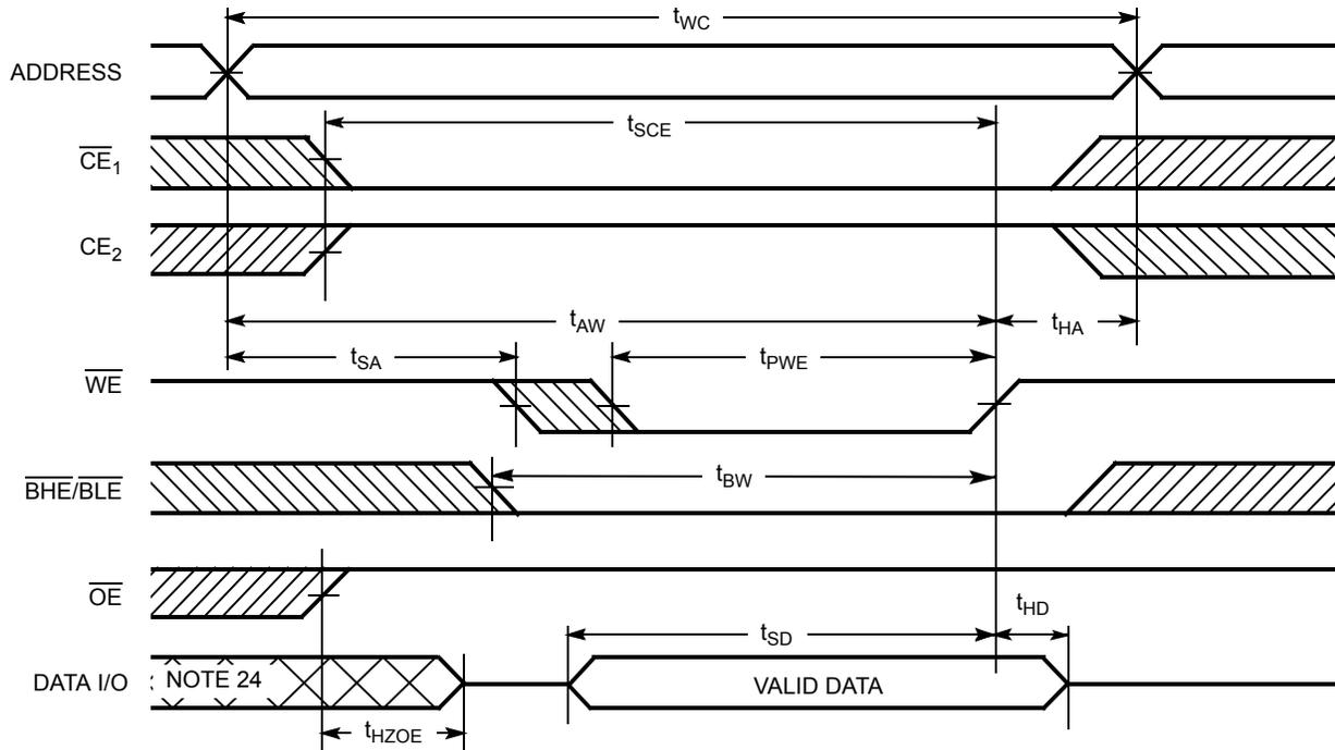
Figure 7. Write Cycle 2:  $\overline{CE}$  Controlled [21, 22, 23]
